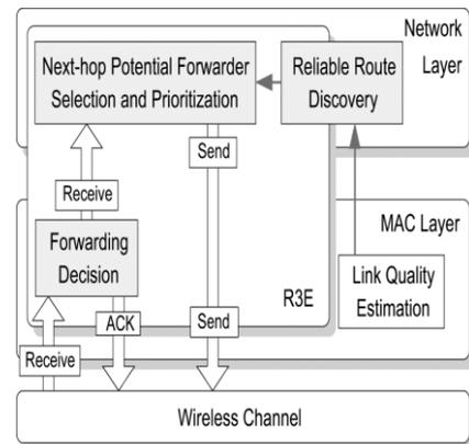
**Fig. 2. Functional architecture overview of up/down stream of reactive protocol**
