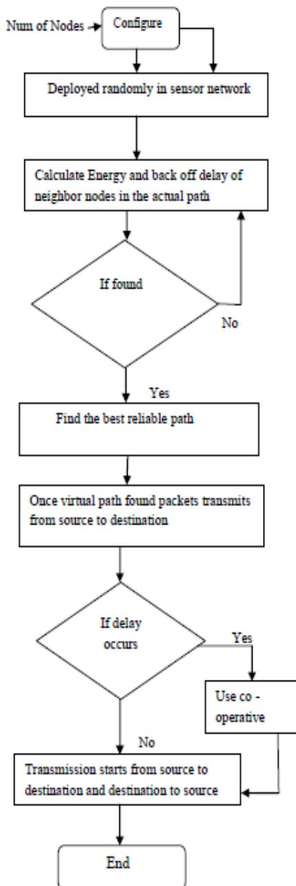
Fig 3: flow chart of packet transmission
