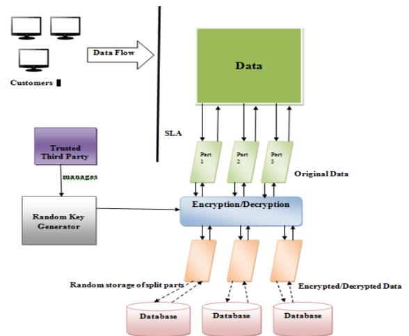
Figure 3:System design for security in Distributed Storage System
