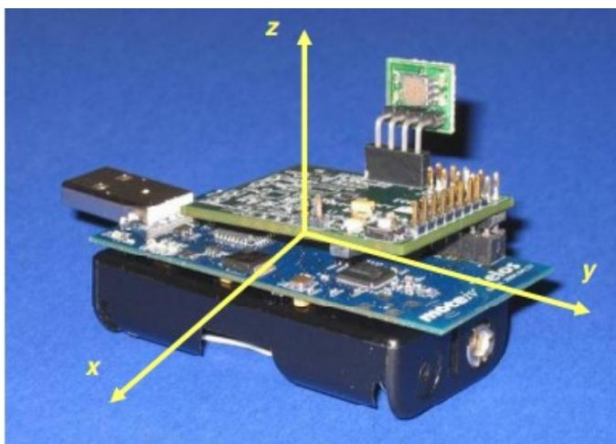
Figure 4. ActiS sensor node – Tmote Sky with ISPM motion sensing daughter card
