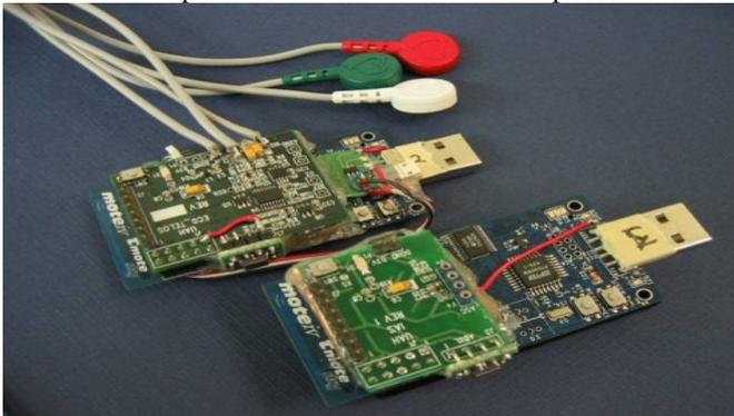
Figure 2. Prototype WBAN sensors. From left to right: eActiS with electrodes, ActiS
