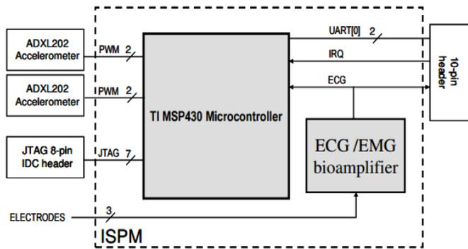
Figure 3. ISPM block diagram
