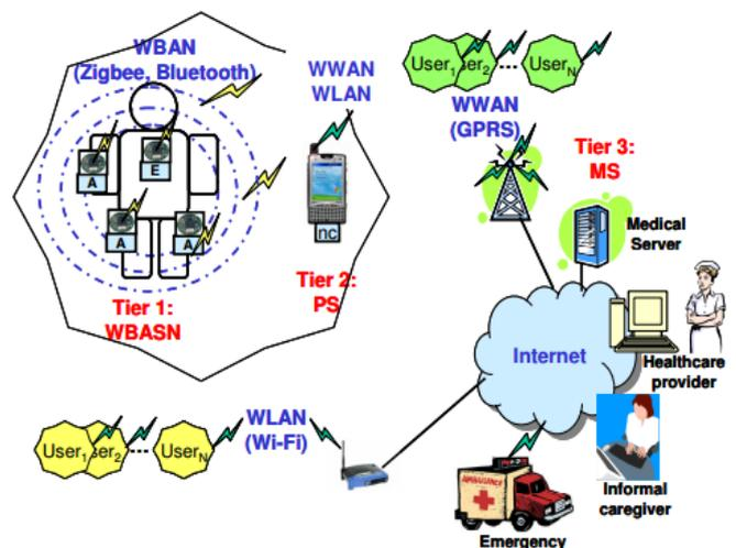
Figure 1. Health monitoring system network architecture
