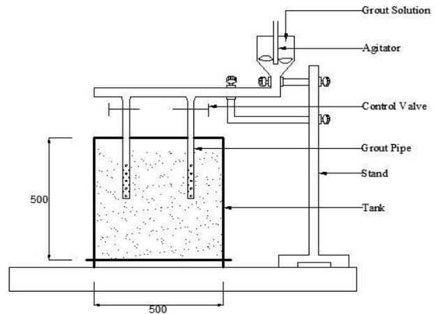
**Fig. 2 Schematic representation of grouting**
