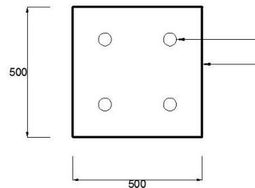
**Fig. 3 Plan view of grout pipes**
