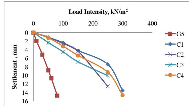
Fig. 6 Plot between load intensity and settlement - grouted soil (Cement grout)
