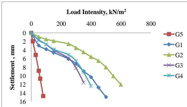
**Fig. 7 Plot between load intensity and settlement - grouted soil (Cement Biopolymer grout)**
