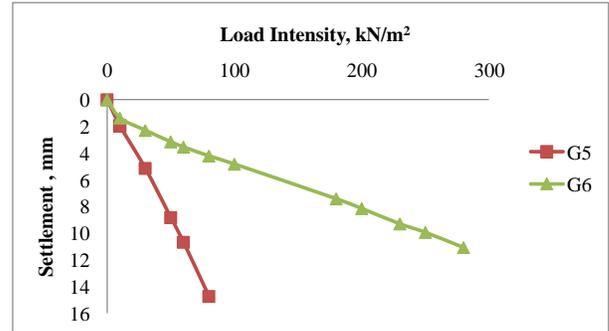
Fig. 5 Plot between load intensity and settlement - ungrouted soil
