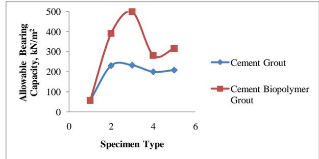
**Fig. 8 Plot between Allowable Bearing capacity (10 mm settlement) and Specimen type**
