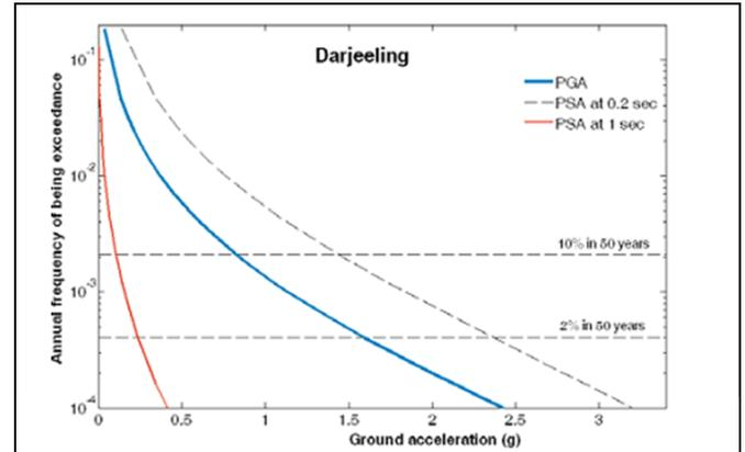
Fig. 1. Seismic hazard curve of the Darjeeling region [4]
