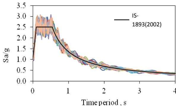
Fig 2. Response Spectra for 44 converted ground motions along with IS 1893 (2002) design spectrum
