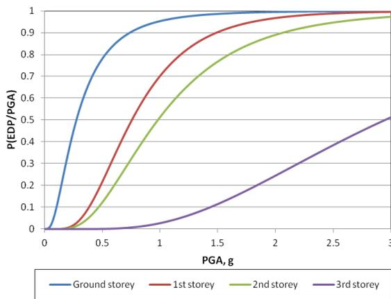
a) Fragility Curve for 4S4B IO performance level for different storey levels
