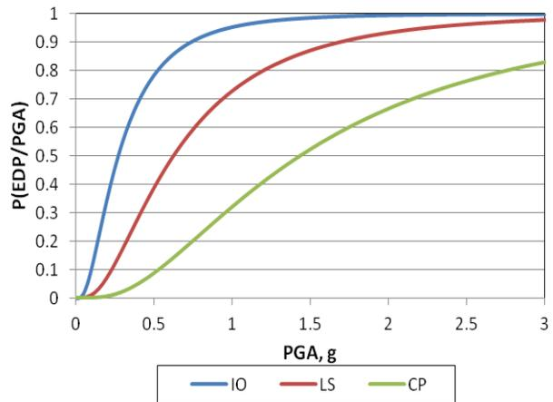
b) Fragility Curve for 4S4B performance levels for Ground Storey
