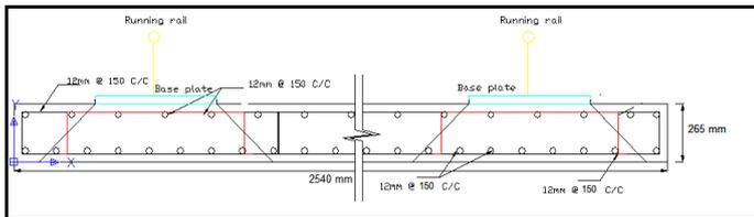
Fig. 14 Reinforcement details of track slab
