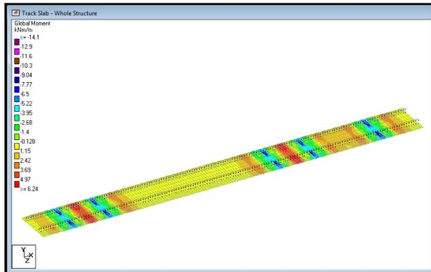
Fig. 12(a) Stress contour in X-direction
