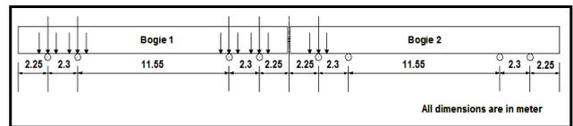
Fig. 7 Diagrammatic representation of bogie details
