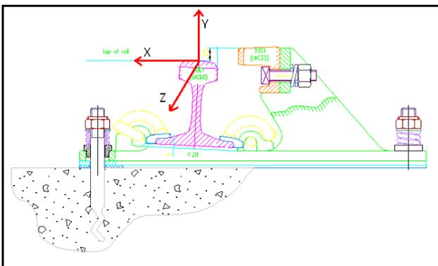
Fig. 6 Axis convention at the top of rail
