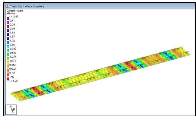
Fig. 11(b) Stress contour in Z-direction
