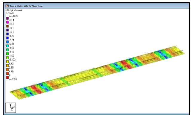
Fig. 11(a) Stress contour in X-direction
