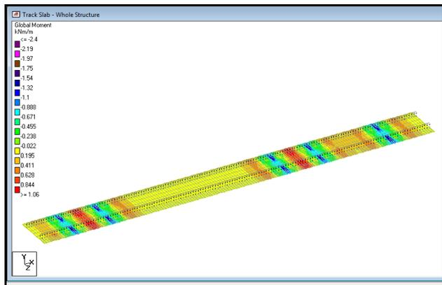
Fig. 12(b) Stress contour in Z-direction
