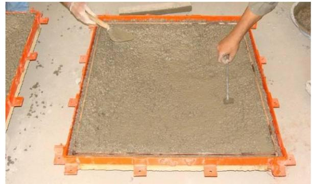
Fig.3 Casting of shell specimen
