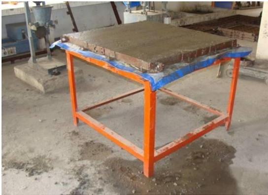
Fig.1 Rectangular steel frame with poly urethane membrane for casting the pre mould
