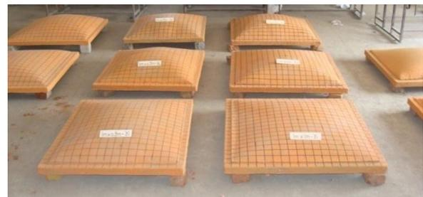
Fig.4 Shell specimens with various rises
