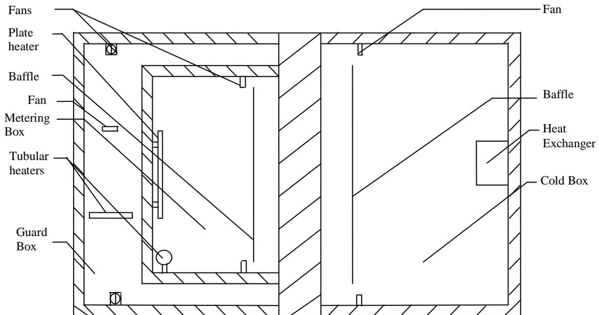
Fig.1. Guarded Hot Box U-value Test Setup
