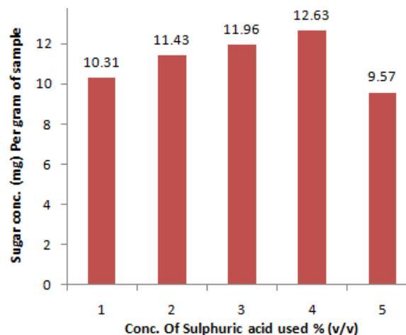
Fig 8: Sugar yield by using different concentrations of sulphuric acid.
