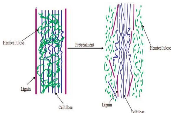
Fig 2: Schematic of the role of pretreatment in the conversion of biomass to fuel. [3]
