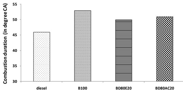
Fig. 9: Combustion duration for the tested fuels at full load
