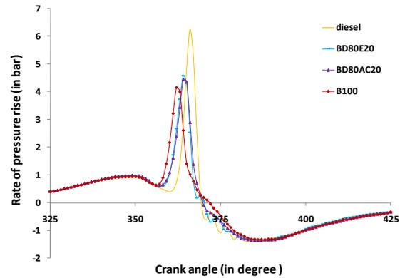
Fig. 4: Rate of pressure rise for the tested fuels.
