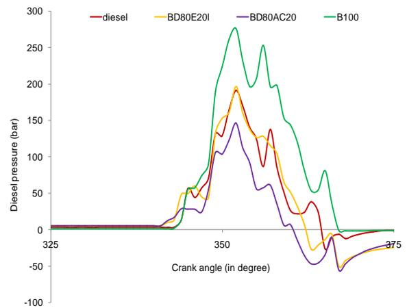
Fig. 7: Fuel line pressure variation with CA for the tested fuels
