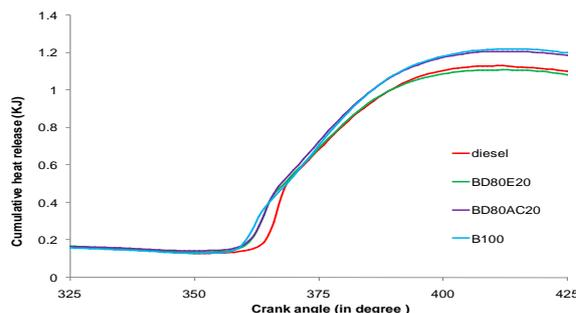
Fig. 6: CHR vs. CA for the tested fuels at full load
