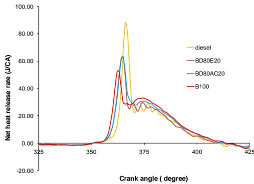
Fig. 5: NHRR vs. CA for the tested fuels at full load
