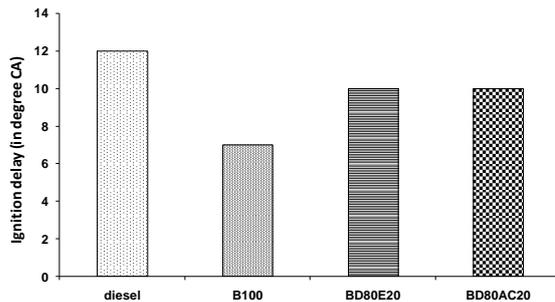
Fig.8: Ignition delay of various fuels at full load
