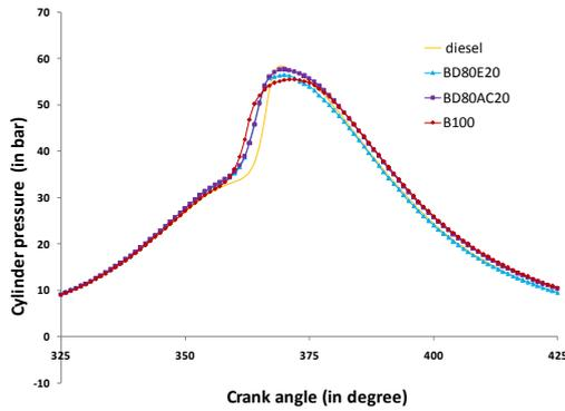
Fig. 2: Cylinder pressure variation for the tested fuels
