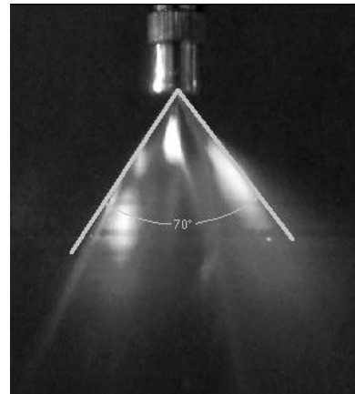
Fig.3. Picture showing cone angle of sunflower oil issued from hollow cone nozzle at 75°C and 3 bar pressure.
