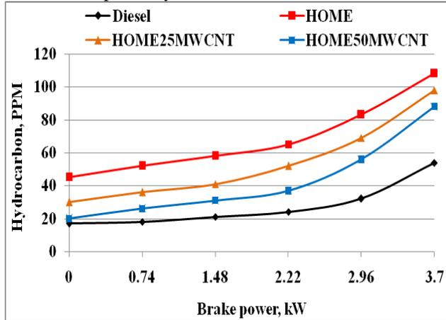
Fig. 4 Variation of hydrocarbon with brake power
