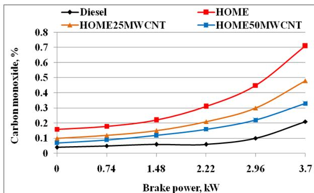
Fig. 5 Variation of carbon monoxide with brake power
