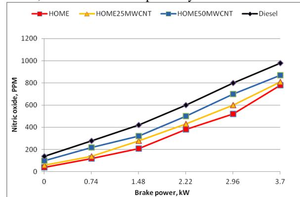
Fig. 6 Variation of nitric oxide with brake power
