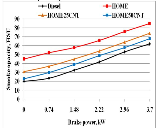
Fig. 3 Variation of smoke opacity with brake power
