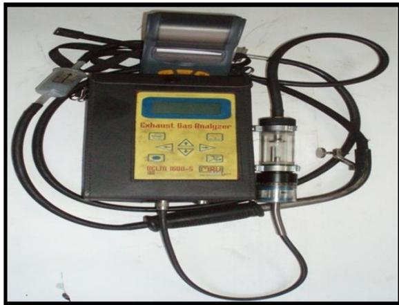
Fig 2: Exhaust Gas Analyzer
