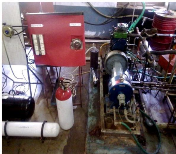
Fig 1.CNG/HCNG-HOME dual fuelled C I engine test rig
