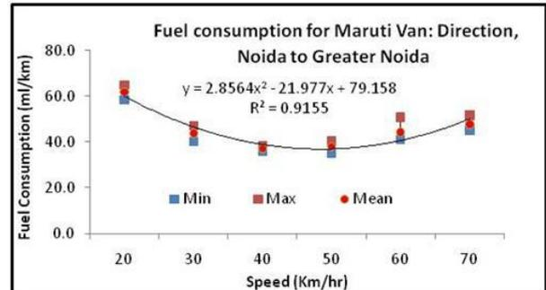
Fig.4. Fuel Consumption of Maruti Van: (Direction: Noida to Greater Noida)
