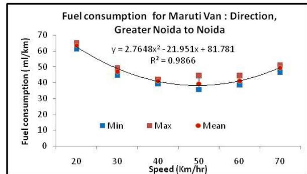
Fig.5. Fuel Consumption of Maruti Van: (Direction: Greater Noida to Noida)
