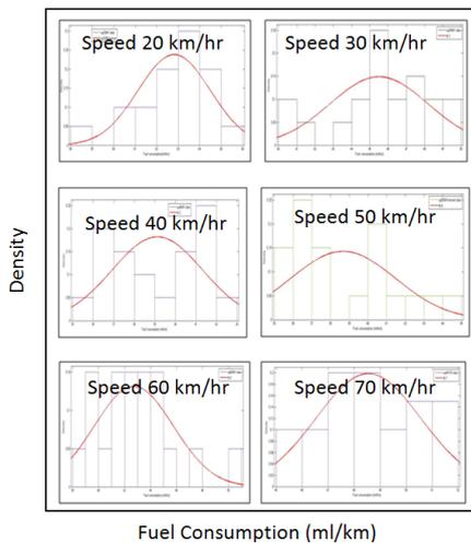
Fig. 6. Probability Distribution of Fuel Consumption for different Steady Speeds of Maruti Van
