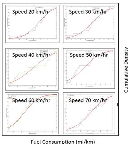
Fig. 7. Cumulative Distribution of Fuel Consumption for different Steady Speeds of Maruti Van
