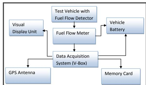
Fig.1. Fuel Flow Data Acquisition System
