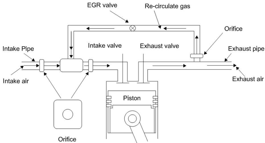
Fig.1. General View of Exhaust Gas Recirculation Technique
