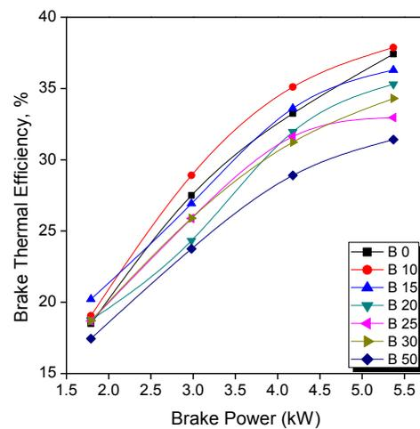
Fig.4. Effect of Brake Power on Brake thermal efficiency for with EGR condition.
