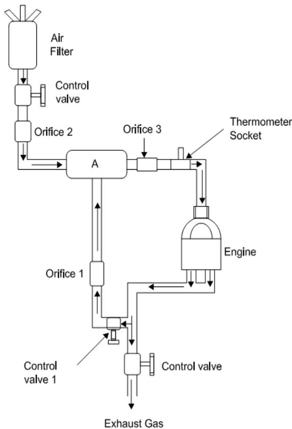
Fig.2. Schematic Diagram of Exhaust Gas Recirculation Setup
