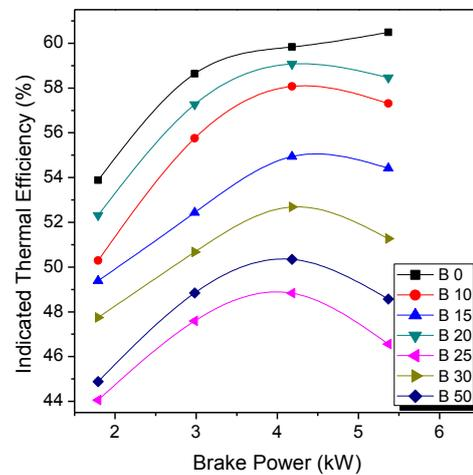
Fig.7. Effect of Brake Power on Indicated thermal efficiency for without EGR condition.
