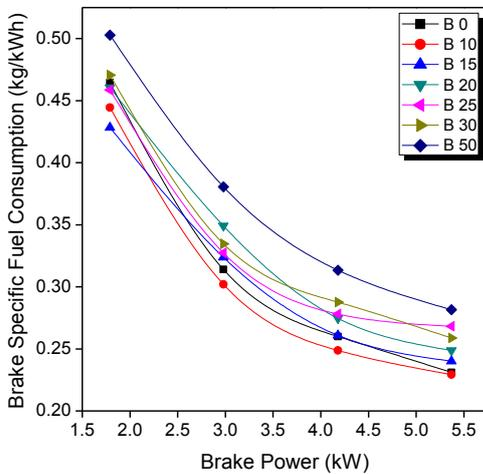
Fig.5. Effect of Brake Power on Brake specific fuel consumption for without EGR condition.
