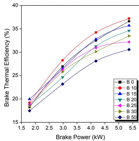
Fig.3. Effect of Brake Power on Brake thermal efficiency for without EGR condition.
