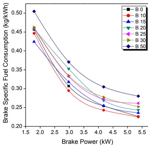
Fig.6. Effect of Brake Power on Brake specific fuel consumption for with EGR condition.
