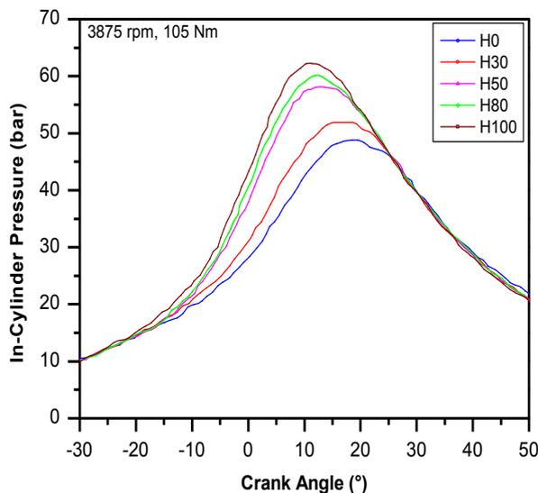
Fig. 4. In-cylinder pressure versus crank angle for 105 N m at 3875 rpm. Source: Melo et al. [21]
