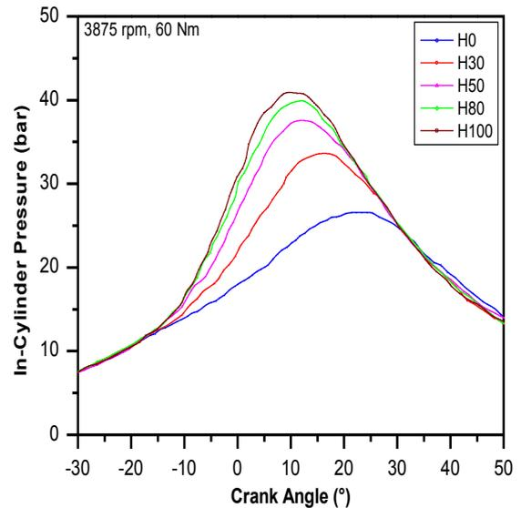
Fig. 5. In-cylinder pressure versus crank angle for 60 Nm at 3875 rpm. Source: Melo et al. [21]
