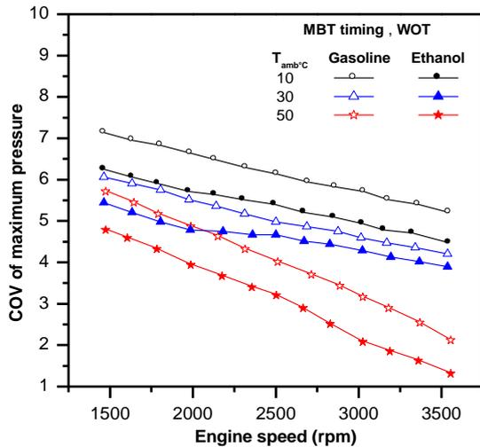
Fig. 1. Coefficient of variation of maximum pressure with intake air temperature. Source: Yoon and Lee [16]
