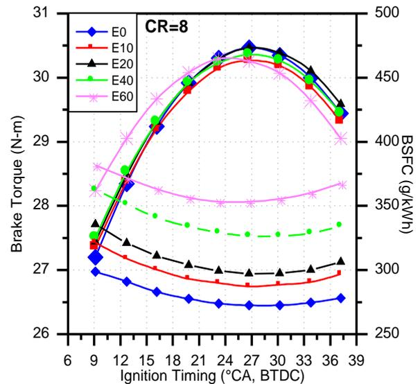
Fig. 2. Variation of engine torque and BSFC with ignition timing at CR=8:1.
