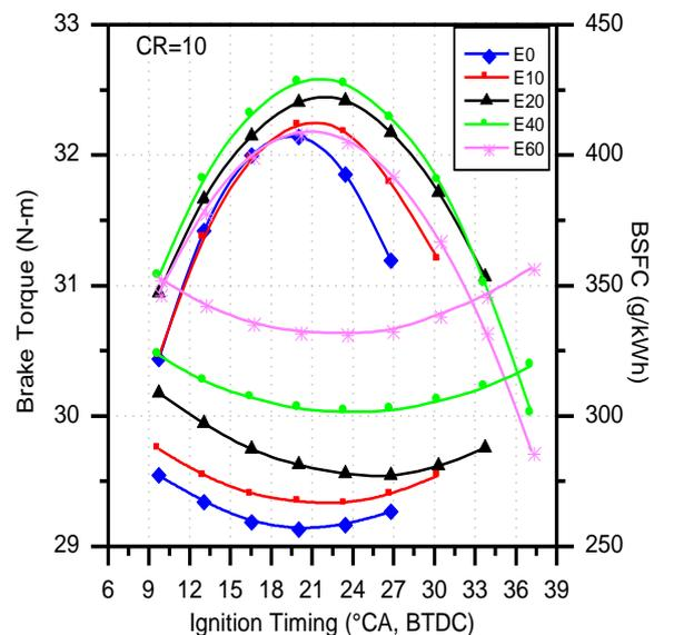
Fig. 3. Variation of engine torque and BSFC with ignition timing at CR=10:1. Source: Topgul et al. [18]
