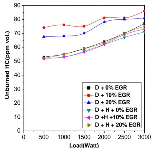
Figure 8: Variation of Unburned Hydrocarbon vs load [6]
