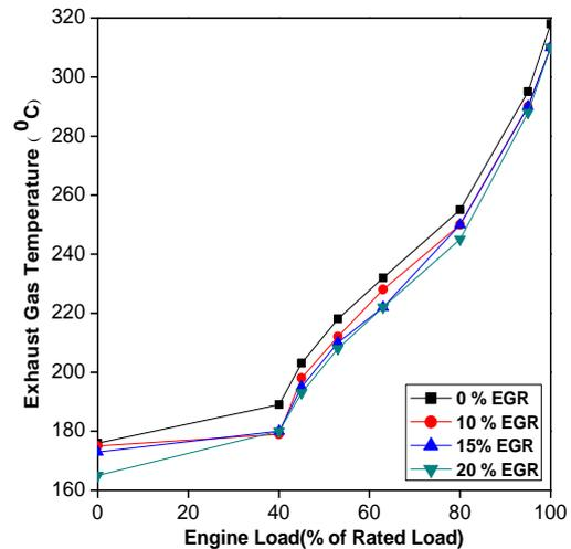
Figure 3: Variation of Exhaust gas Temperature vs Load [4]
