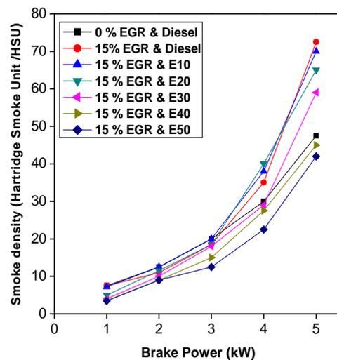
Figure 4: Variation of Smoke Density vs Brake Power [7]
