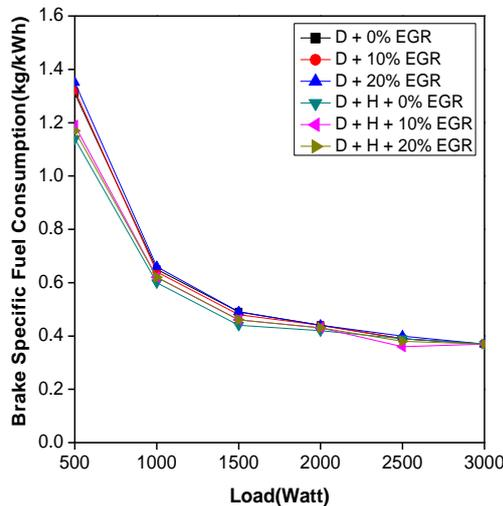
Figure 1: Variation of Brake Specific Fuel Consumption vs Load [6]
