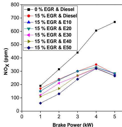
Figure 6: Variation of NO<sub>x</sub> vs Brake Power [7]
