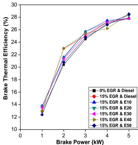
Figure 2: Variation of Brake Thermal Efficiency vs Brake Power [7]
