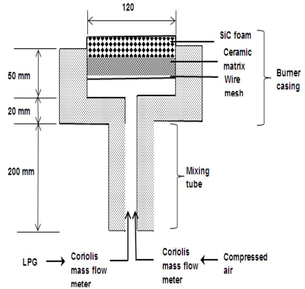
Fig. 2. Schematic of porous radiant burner (PRB).
