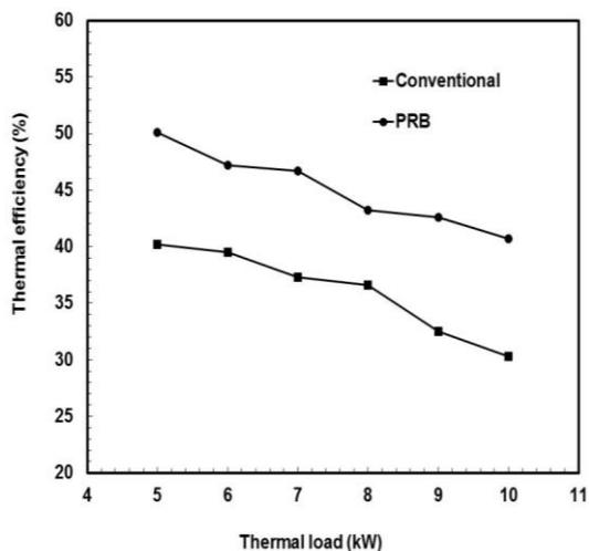
Fig. 4. Thermal efficiency of different burners.
