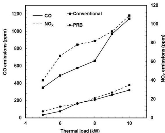
Fig. 5. Comparison of CO and NOx emissions for different thermal loads for PRB with conventional burner.
