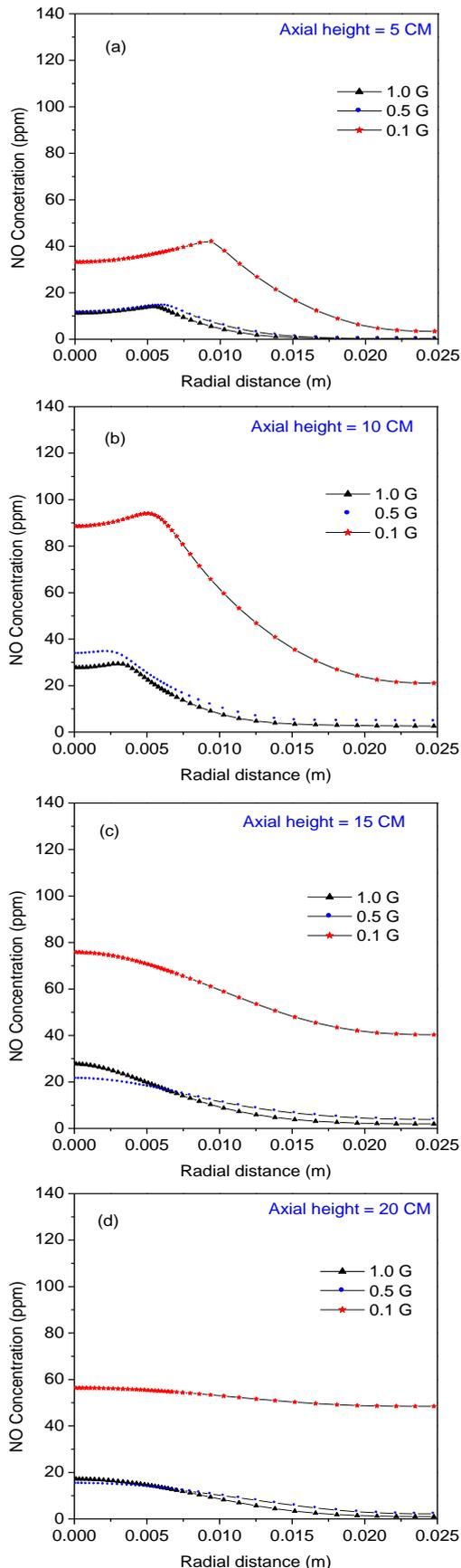
**Fig. 5** Radial distributions of NO concentration at different axial heights: (a) 5 cm (b) 10 cm (c) 15 cm and (d) 20cm
