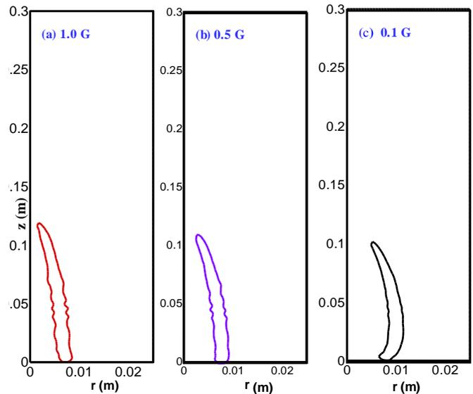
**Fig. 2** Shape of the flame fronts for three different gravity levels: (a) 1.0 G, (b) 0.50 G and (c) 0.10 G
