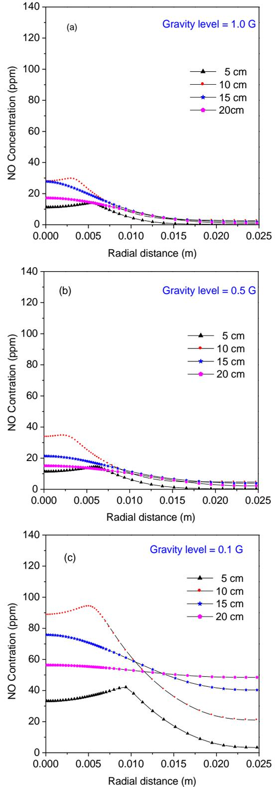
**Fig. 4.** Radial distributions of NO concentration at different axial planes, for gravity levels: (a) 1.0 G, (b) 0.50 G and (c) 0.10 G
