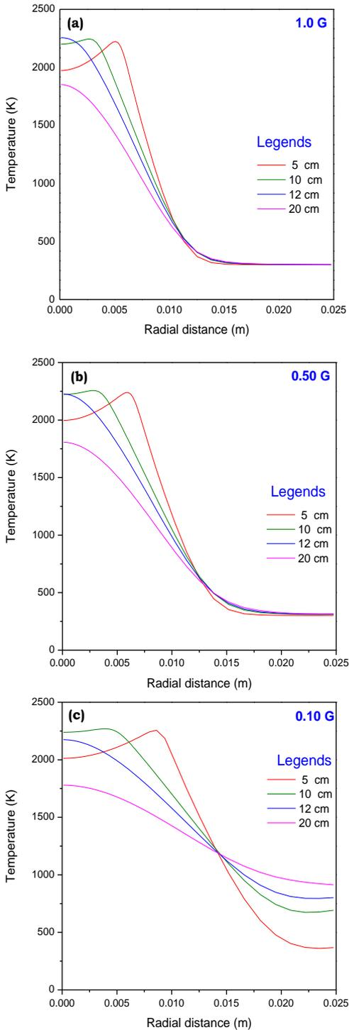
**Fig. 3.** Radial distributions of temperature at different axial planes, for three gravity levels: (a) 1.0 G (b) 0.50 G and (c) 0.10 G
