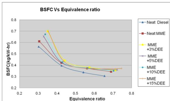
Fig. 8 Brake Specific Fuel Consumption Vs Equivalence ratio graph with different percentages of additive Diethyl Ether (DEE)
