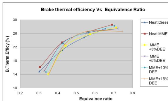
Fig.9 Brake Thermal Efficiency Vs Equivalence Ratio graph with different percentages of additive Diethyl Ether (DEE)
