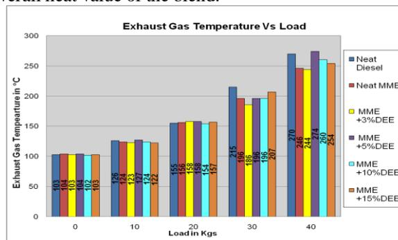
Fig.10 Exhaust Gas Temperature Vs Load Graph with different percentages of (DEE) along with Biodiesel at all loads.
