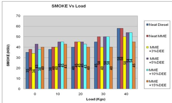
Fig.11 Smoke Vs Load Graph with different percentages of (DEE) along with Biodiesel at all loads
