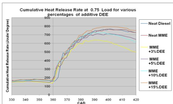
Fig.7 Cumulative heat release rate comparison with various percentages of Additive Diethyl Ether (DEE) along with Biodiesel at 3/4<sup>th</sup> Full Load.
