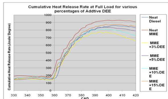
Fig.6 Cumulative heat release rate comparison with various percentages of Additive Diethyl Ether (DEE) along with Biodiesel at Full Load.
