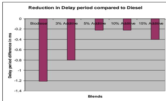
Fig.12 Delay period difference in milliseconds w.r.t. Diesel at full load.
