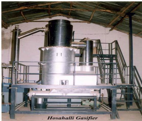
Fig 3(a) : Biomass Gasification System (20 kWe) at Hosahalli, Karnataka [27].
