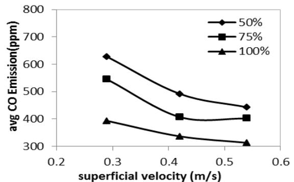
Fig. 2. Effect of Superficial Velocity and Biomass Content to the Average of CO Emissions
