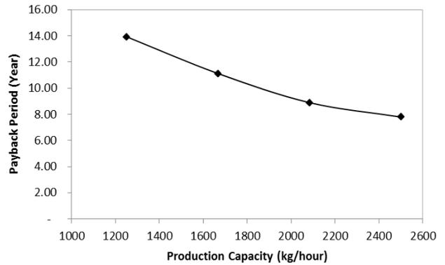
Fig. 7. Payback Period per Production Capacity
