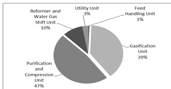
Fig. 4. Bare Module Equipment Cost Breakdown
