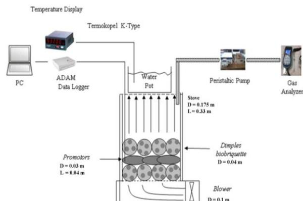
Fig.1. The Experimental Set Up with Data Collection Scheme
