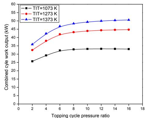
Fig.2. Variation of combined cycle work output with topping cycle pressure ratio.
