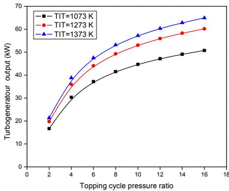
Fig.3. Variation of turbo generator work output with topping cycle pressure ratio.
