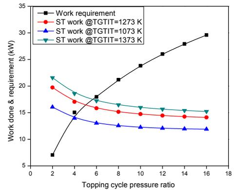
Fig.5. Variation of work done and work requirement of different components with topping cycle pressure ratio.
