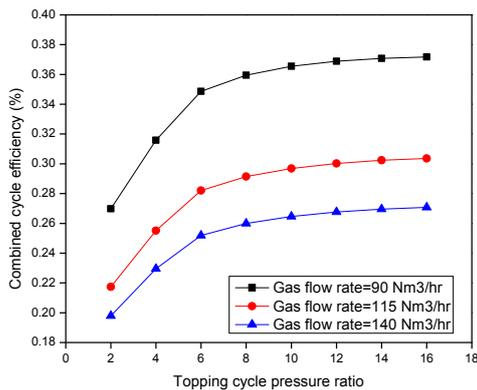
Fig.7. Variation of combined cycle efficiency with topping cycle pressure ratio (TIT=1273K).
