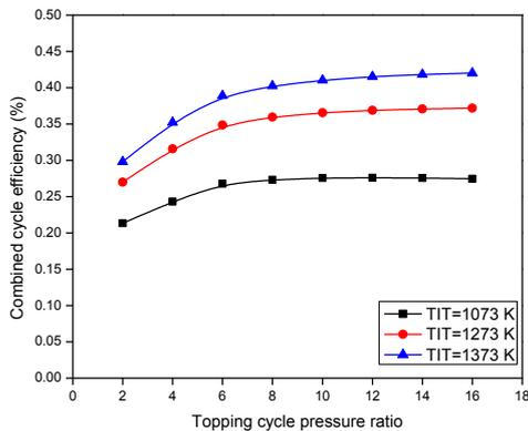
Fig.4. Variation of combined cycle efficiency with topping cycle pressure ratio.
