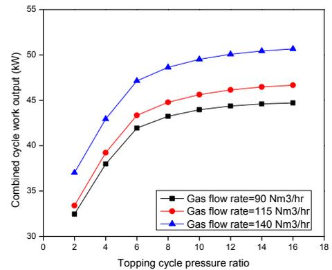
Fig.6. Variation of combined cycle work output with topping cycle pressure ratio (TIT=1273K).
