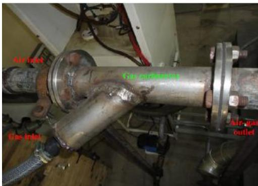
Fig. 2 T-junction gas mixer developed by Sahoo [4]
