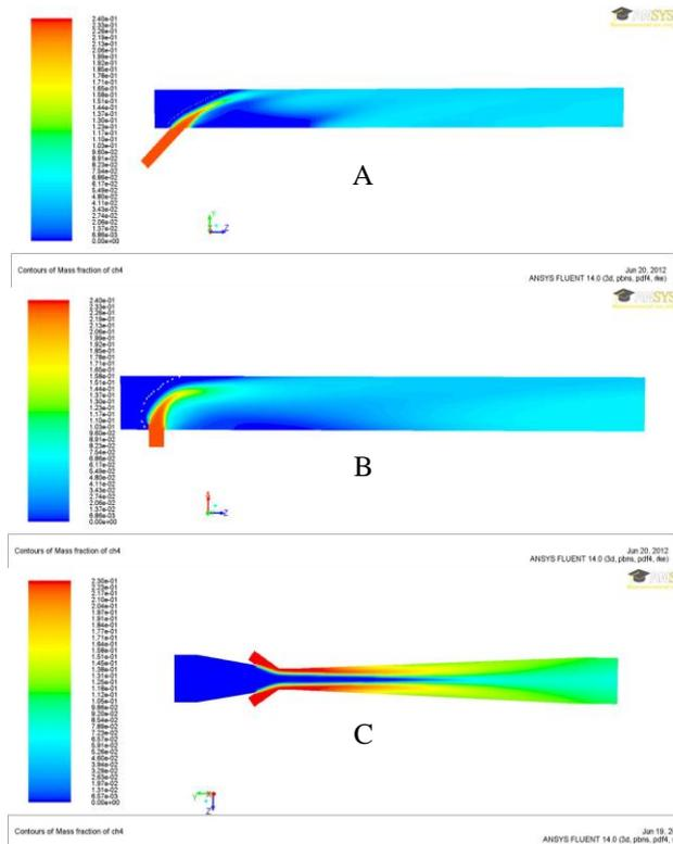
Fig.8 CH<sub>4</sub> contour of (A) existing T-junction design gas mixer, single nozzle inclined at an angle of 45° (B) contour of existing T-junction design gas mixer, single nozzle inclined at an angle of 90°(C) venturi gas mixer
