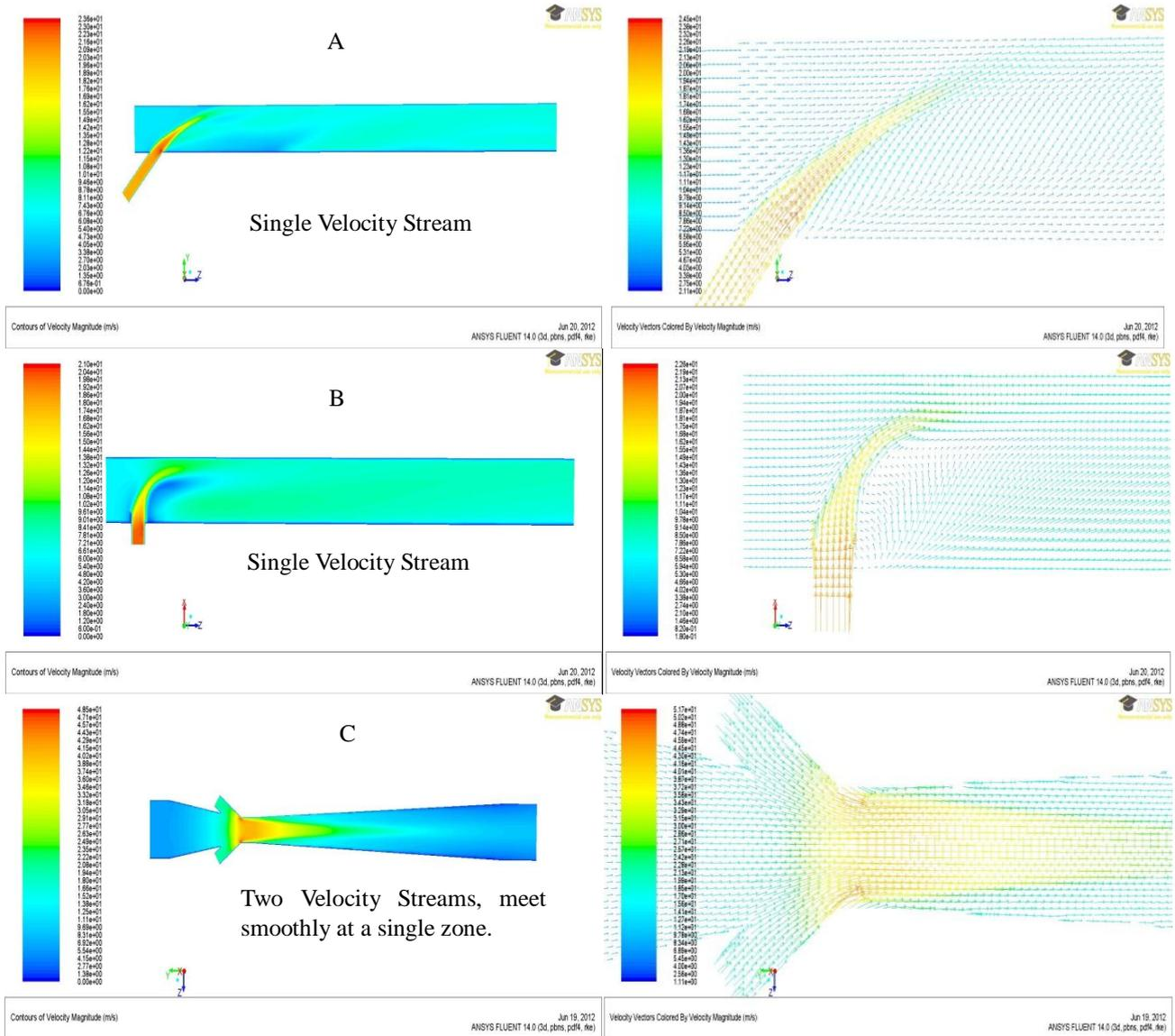
Fig.7 Velocity and Velocity Vector contour of (A) existing T-junction design gas mixer, single nozzle inclined at an angle of 45°(B) existing T-junction design gas mixer, single nozzle inclined at an angle of 90° (C) venturi gas mixer
