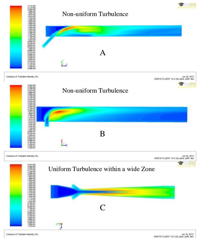
Fig.6 (A) Turbulence contour of existing T-junction design gas mixer, single nozzle inclined at an angle of 45° (B) Turbulence contour of existing T-junction design gas mixer, single nozzle inclined at an angle of 90°, and (C) Turbulence contour of venturi gas mixer
