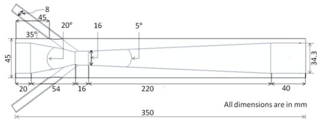
Fig. 4 The schematic diagram of the venturi gas mixer
