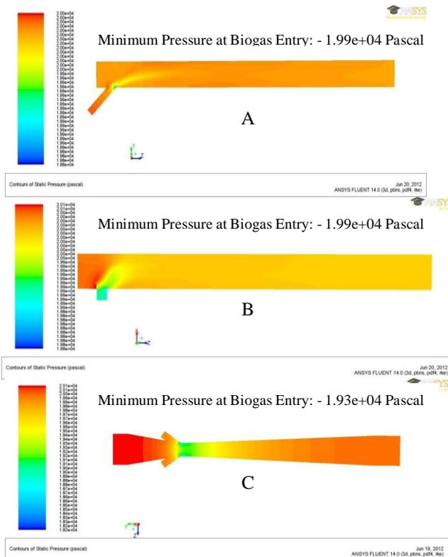
Fig.5 (A) Pressure contour of existing T-junction design gas mixer, single nozzle inclined at an angle of 45°, (B) Pressure contour of existing T-junction design gas mixer, single nozzle inclined at an angle of 90°(C) Pressure contour of venturi gas mixer
