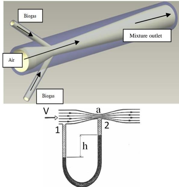
Fig. 3 Proposed design of venturi gas mixer
