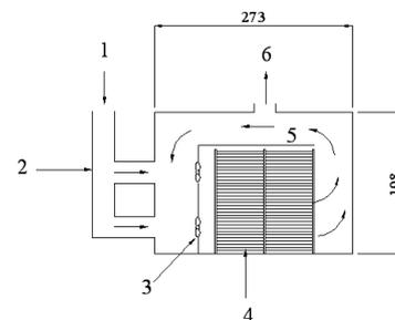
1. Hot air from solar collector 2. Insulated duct 3. Axial fans 4. Perforated trays
