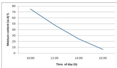
Fig. 4 Reduction in moisture content of the product with time
