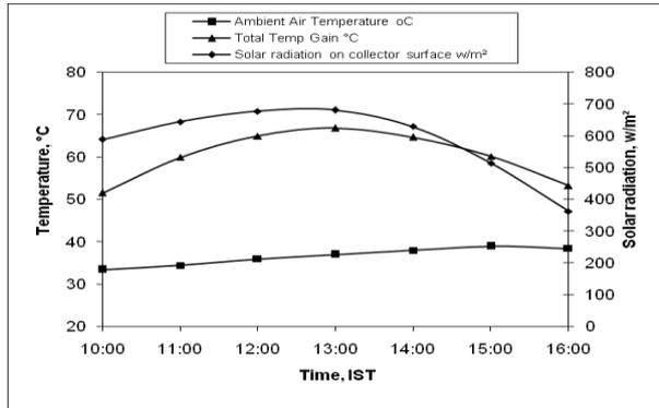
Fig. 3 Variation of temperature outlet of solar air heater with solar radiation
