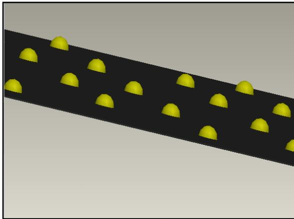
Fig.1 Hemispherical protruded solar energy absorber
