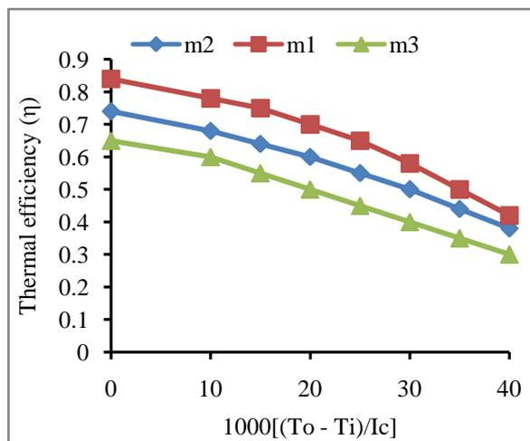
Fig. 6 Variations of collector efficiency with temperature parameter for pin fin absorber.
