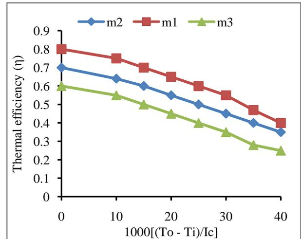
Fig. 7 Variations of collector efficiency with temperature parameter for hemispherical protrusion.
