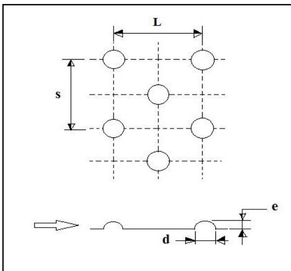
Fig.2 Long way and short way length of absorber
