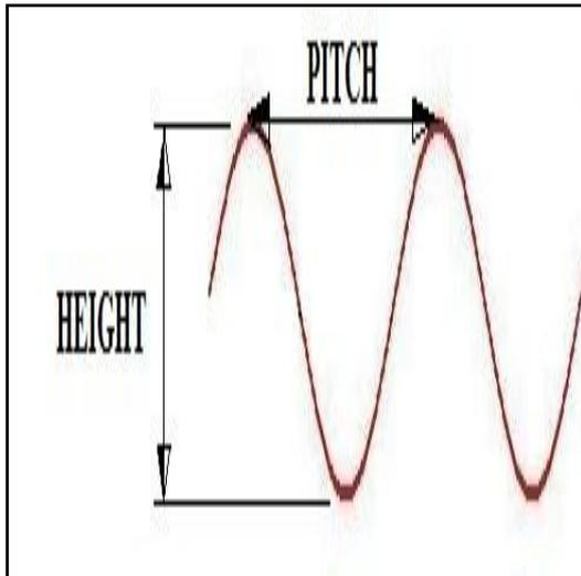
Fig.5 Profile of corrugated absorber
