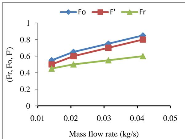
Fig.10 Heat gain factor for hemispherical absorber
