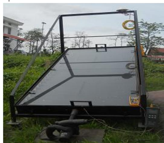
Fig.4 Sine wave corrugated solar air heater
