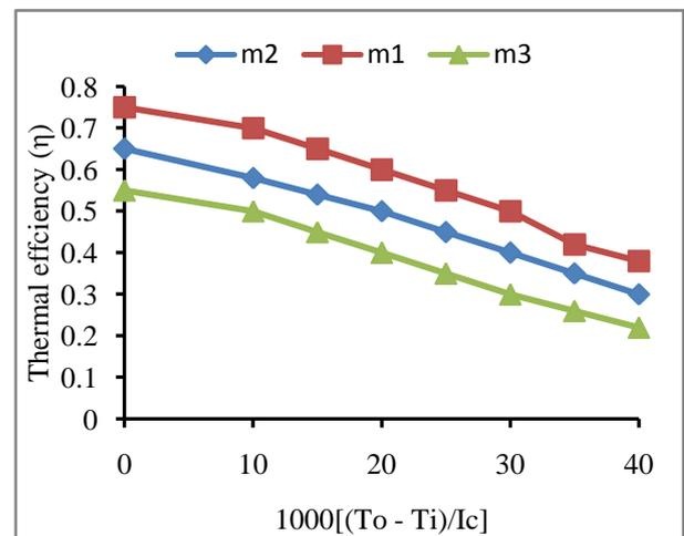
Fig. 8 Variations of collector efficiency with temperature parameter for corrugated absorber
