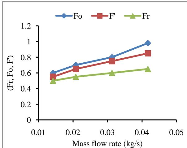
Fig.9 Heat gain factor for pin fin
