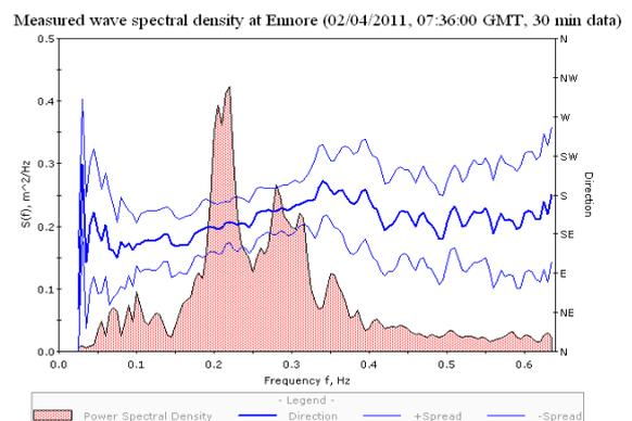
Fig 6.2 Collected WRB data spectrum
