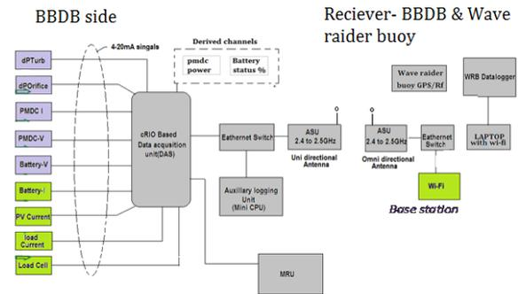
Fig 5.3 Integration of BBDB Instruments with DAS
