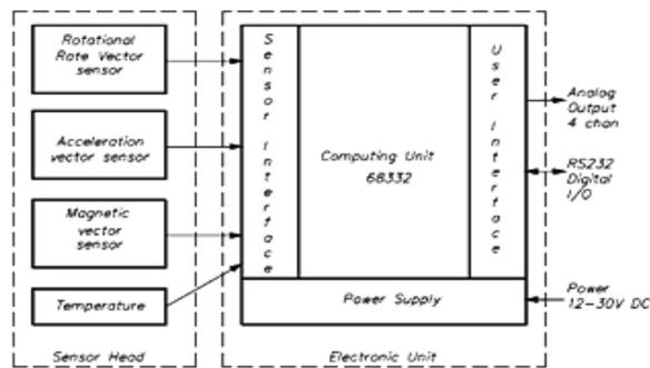
Fig 6.1 Internal block diagram of MRU
