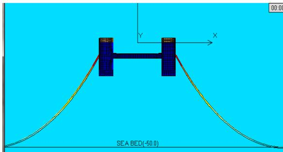
**Figure.5 AQWAGS image of moored semisubmersible**
