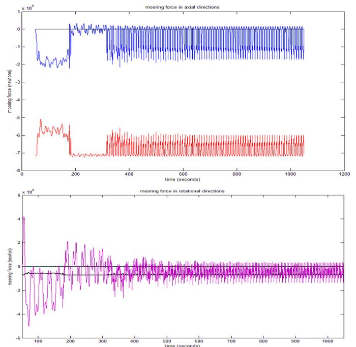
**Figure 6 Mooring force variation in axial and rotational directions**
