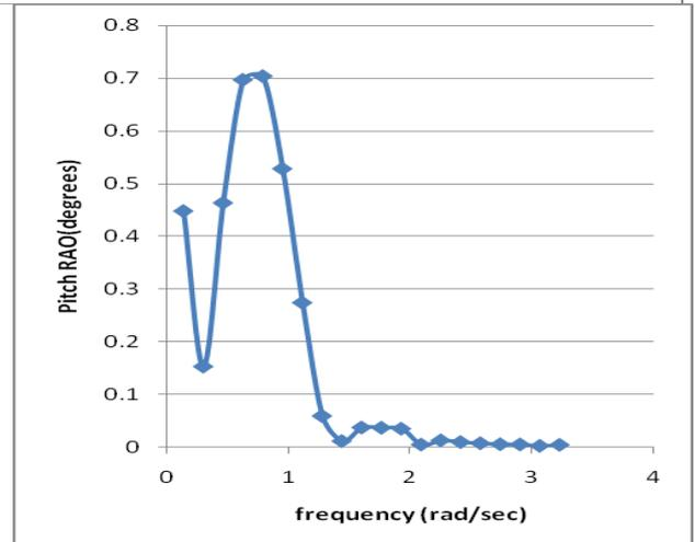
**Figure 3 RAO of semisubmersible for 0degree wave heading**
