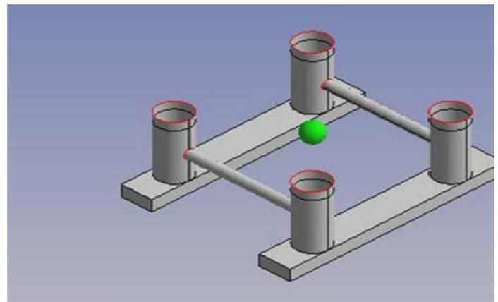
**Figure 2 ANSYS AQWA model of semisubmersible**
