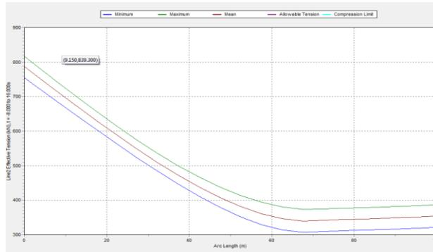
Figure 7 Tension along the mooring line
