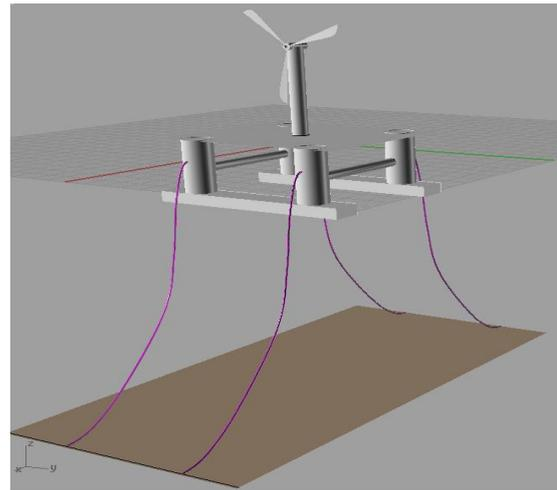
**Figure 1. wind turbine model**
