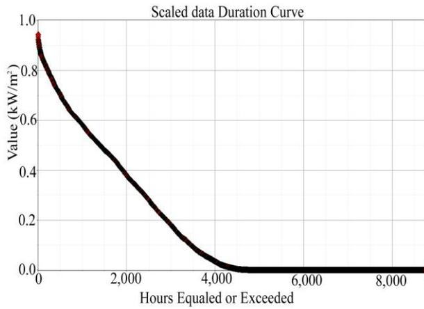
Figure 2: Global Solar radiation duration during a year
