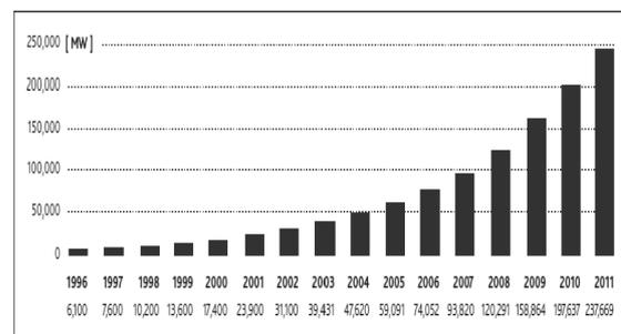
Fig.1 World cumulative wind power installed capacity (1996–2011)
