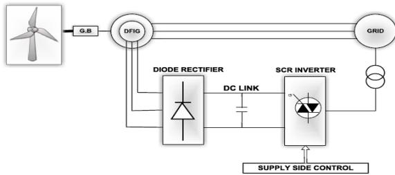
Fig.9 Schematic of static Kramer drive
