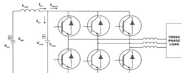
Fig.11. Resonant DC-link Converter
