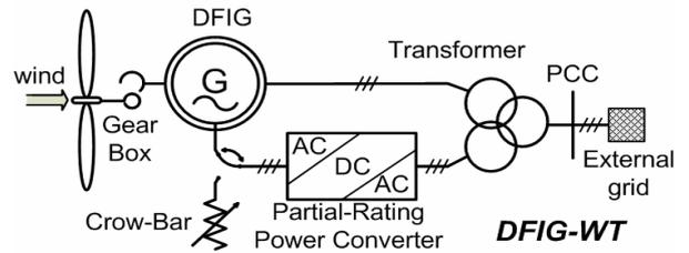
Fig 6. Variable speed WT with partial scale power converter
