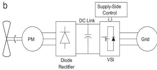
Fig. 14. Block diagram of hard switching supply side inverter
