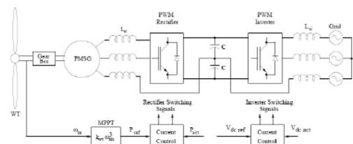
Fig.16. Schematic Diagram of Back-Back PWM converter
