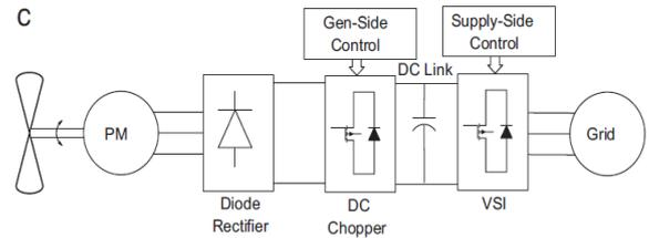
Fig: 15. Intermediate DC/DC converter stage
