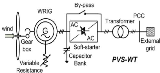
Fig. 5. Partial variable speed WT with variable rotor resistance
