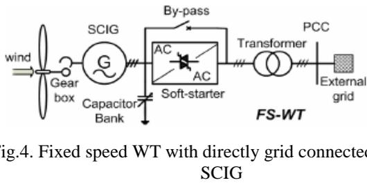
Fig.4. Fixed speed WT with directly grid connected SCIG
