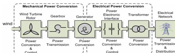
Fig.3. Power conversion stages in a modern WT
