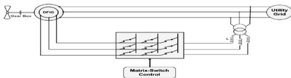
Fig12. Matrix Converter topology with DFIG
