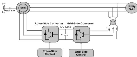
Fig.10. DFIG with back-to-back PWM converter
