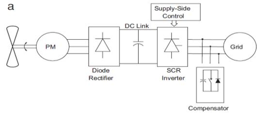
Fig 13. Blok Diagram of Thyristor supply side inverter
