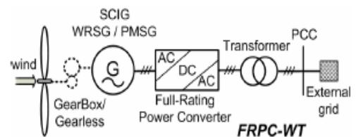
Fig 7 Variable speed WT with full-rating power converter
