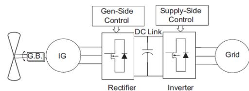
Fig.8. Induction generator with back to back converters
