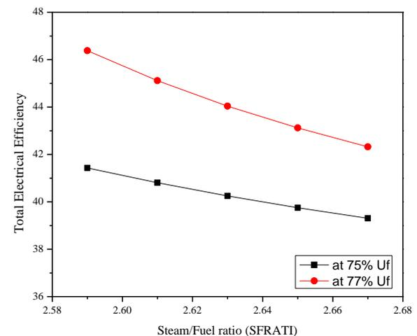
Fig. 4: Variation of total electric efficiency of the hybrid system with SFRATI for fuel utilizations 75% and 77% respectively
