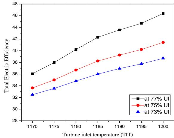
Fig. 2: Variation of total electric efficiency of the hybrid system with turbine inlet temperature for fuel utilizations 73%, 75% and 77% respectively
