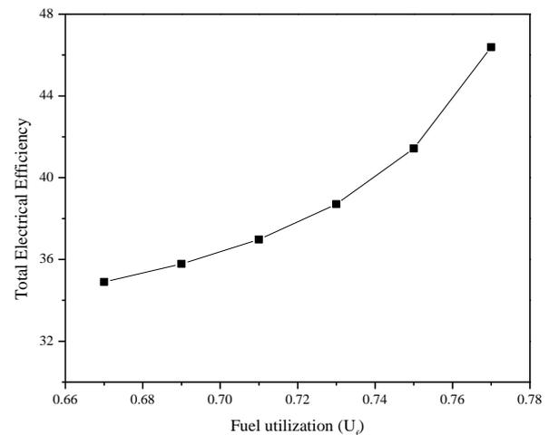
Fig. 3: Variation of total electric efficiency of the hybrid system with fuel utilization for turbine inlet temperature of 1200°C
