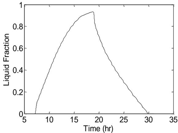
Fig.5. Variation of Melt Fraction of the PCM with time
