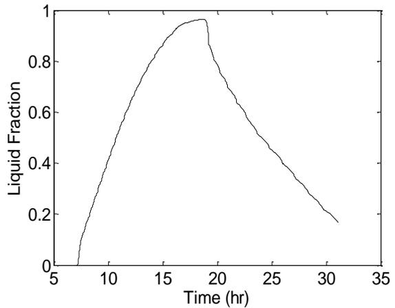
Fig.3. Variation of Melt Fraction of the PCM with time
