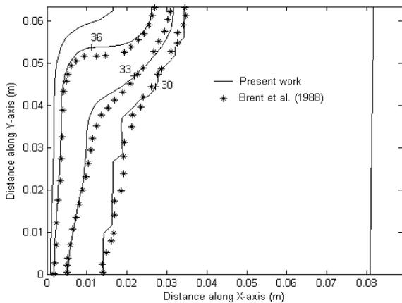
Fig.2. Temperature field at 6min for 2-D melting of gallium
