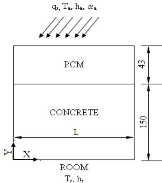
Fig.1. A schematic of the computational domain
