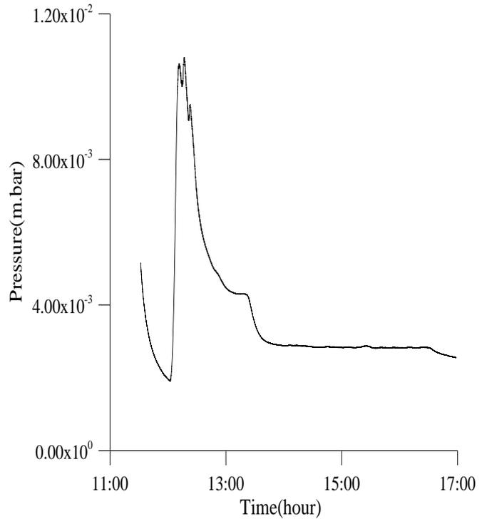
Fig.6 Time-Pressure characteristic curve in vacuum chamber connecting line.
