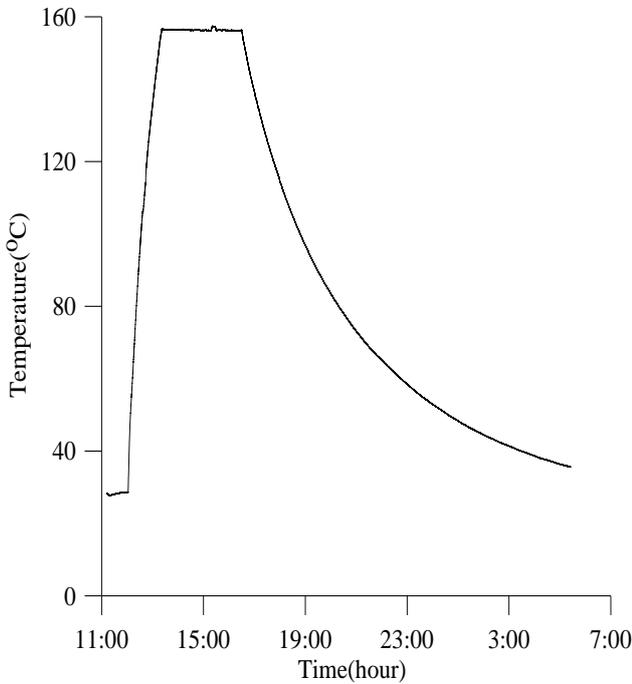
Fig.4 Time-Temperature characteristic curve.
