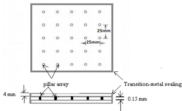
Fig.1 Transition-metal sealed evacuated glazing
