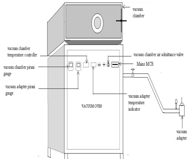
Fig.3 Vacuum oven assembly
