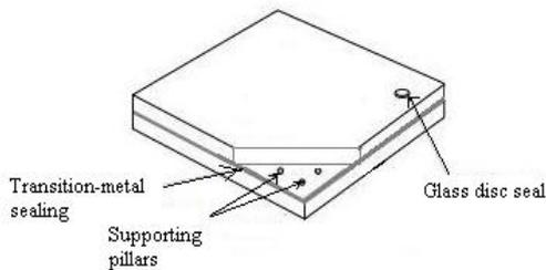
Fig.2 Schematic diagram of an evacuated glazing
