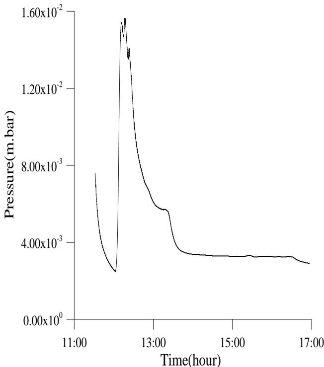
Fig.5 Time-Pressure characteristic curve in vacuum chamber .
