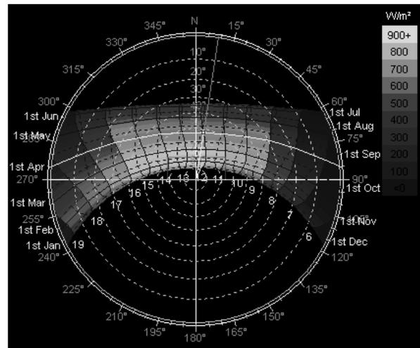
Figure 1 Typical solar chart (sun path diagram)
