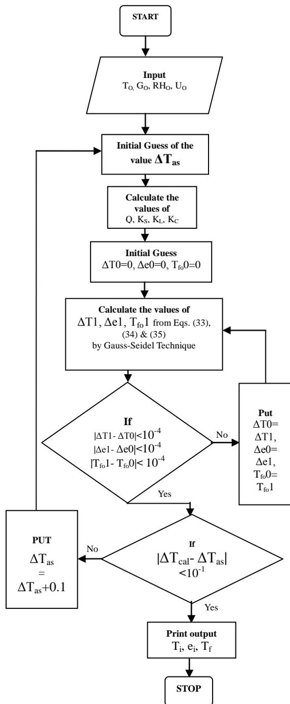
Fig. 2: Flowchart of the developed Thermal Model
