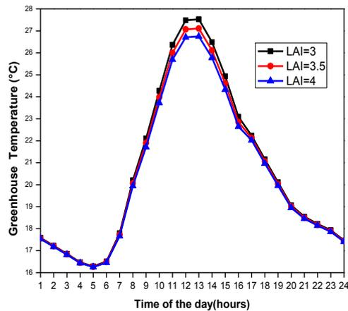
Fig.4: Variation of temperature with time for various LAI
