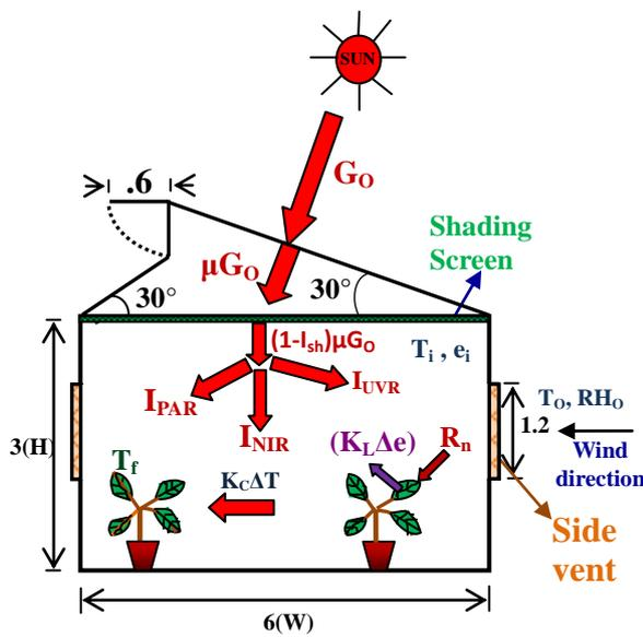
Fig. 1: Energy distribution of greenhouse showing the details of different heat transfer
