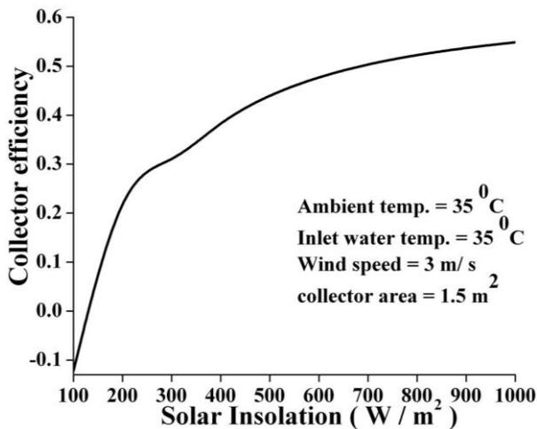
Fig.7. Variation of collector efficiency with solar radiation on fixed date and time
