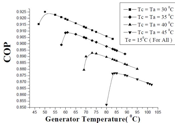
Fig.3. Effect of generator temperature on COP
