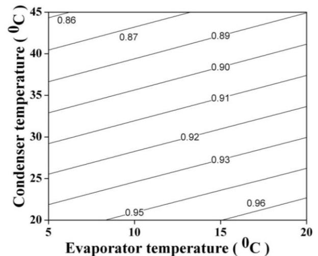
Fig.5. Contour of maximum COP at optimum generator temperature
