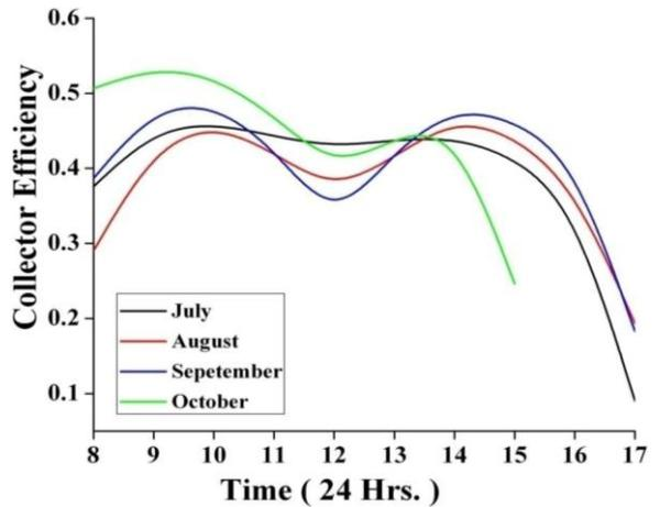
Fig.9. Variation of collector efficiency with respect to time for July to October
