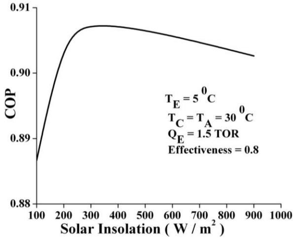
Fig.6. Variation of COP with solar radiation on fixed date and time
