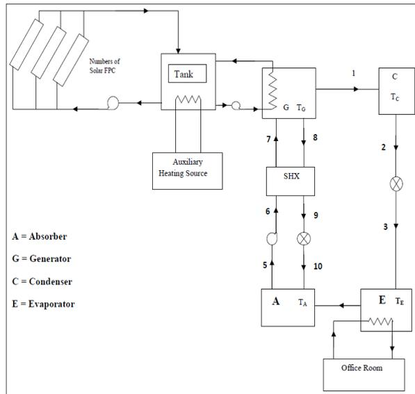
Fig.1. Schematic diagram of complete solar-assisted airconditioning system
