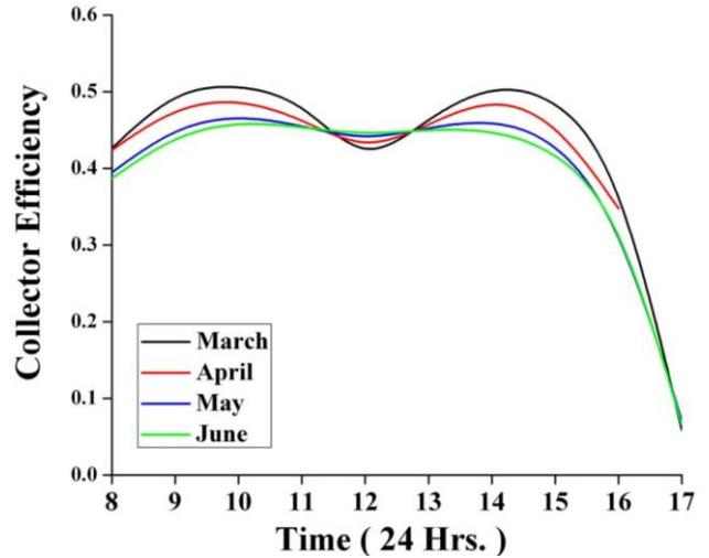
Fig.8. Variation of collector efficiency with respect to time for March to June
