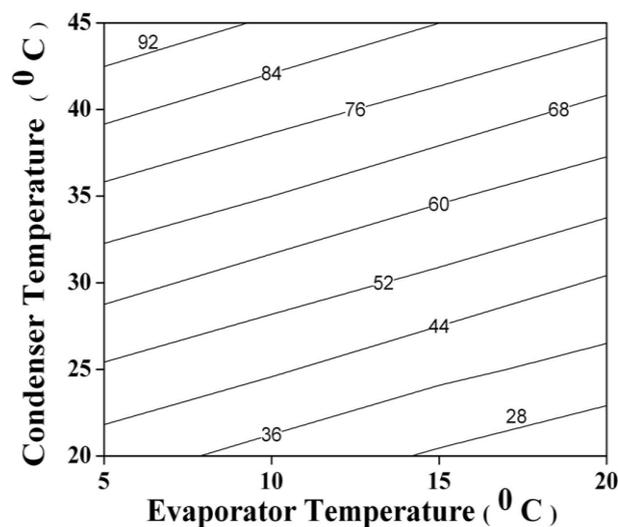
Fig.4. Contour of optimum generator temperature
