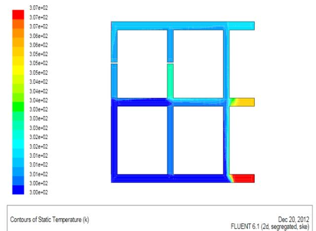
Figure 4: Temperature contour of 2 × 2 Bord and Pillar structure
