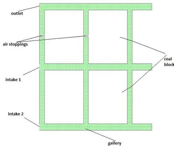
Figure 2: Grid display of 2 × 2 Bord and Pillar structure
