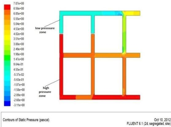
Figure 5: Pressure contour of 2 × 2 Bord and Pillar structure
