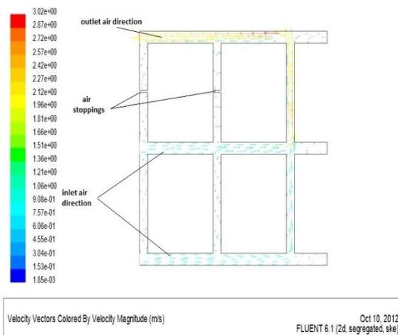
Figure 6: Velocity vector of 2 × 2 Bord and Pillar structure
