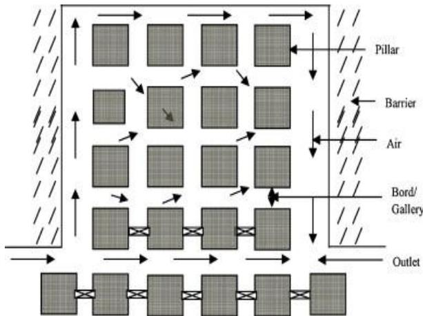
Figure 1: Bord and Pillar structure of coal mine
