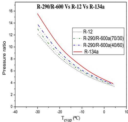
Fig.8 Pressure ratio R-290/R600a vs R-12 vs R-134a
