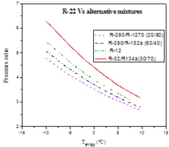
Fig.9 Pressure ratio R-22 vs alternatives
