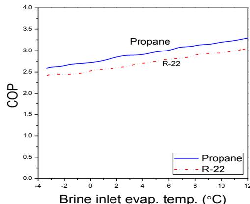
Fig.11. COP of a heat pump with R-22 and R-290, for different brine inlet evaporator
