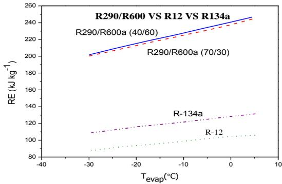
Fig.6 Refrigerating effect R-290 vs R-12 vs R-134a
