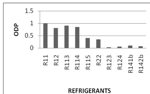
Fig.2. Ozone depletion potential of pure CFC and HCFC refrigerants
