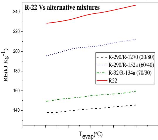
Fig.7 Refrigerating effect R-22 vs alternative mixtures
