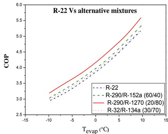
Fig.12. Variation of COP with evaporation temperature for HC mixtures
