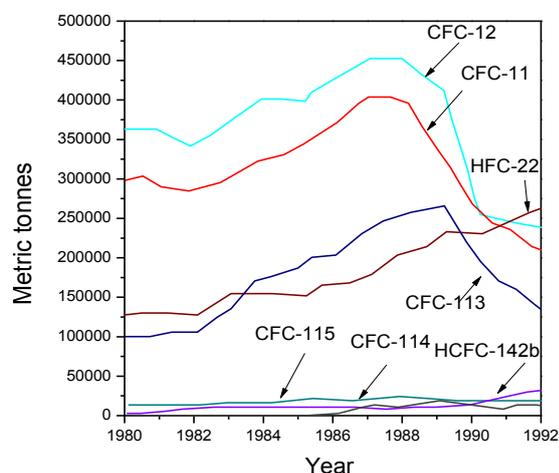
Fig.1. Production of halogenated refrigerants
