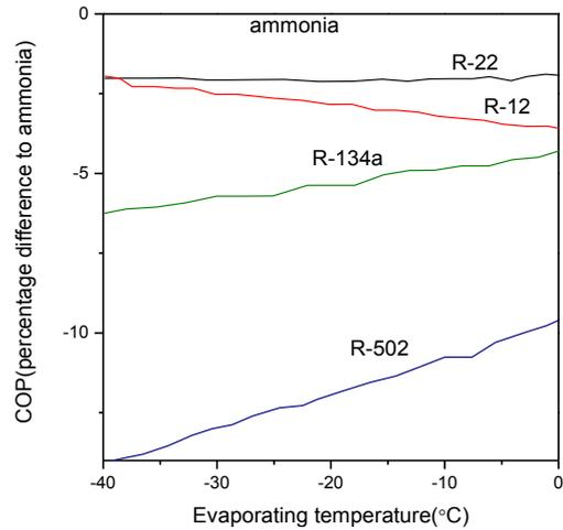
Fig.10. Relative COP of an isentropic vapour compression cycle for different refrigerants [5].
