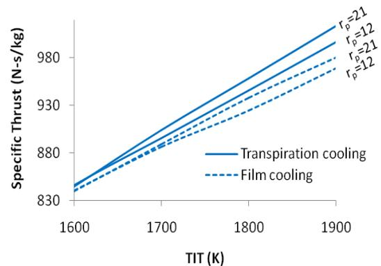
Fig. 2 Variation of Specific thrust with TIT and compressor pressure ratio
