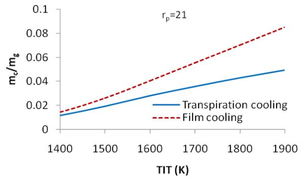
Fig.1. Variation of coolant to gas mass flow ratio with TIT for different cooling techniques
