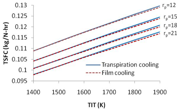
Fig. 3 Variation of thrust specific fuel consumption with TIT and compressor pressure ratio
