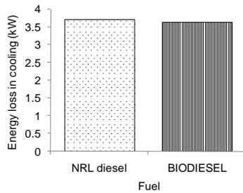
Fig. 8. Cooling loss at full load
