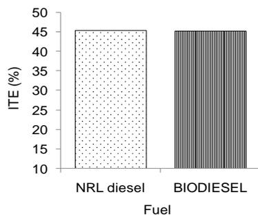
Fig. 5. ITE at full load
