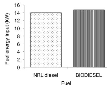
Fig. 7. Fuel energy input at full load
