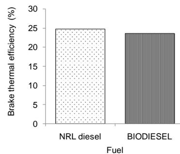
Fig. 2. BTE at full load
