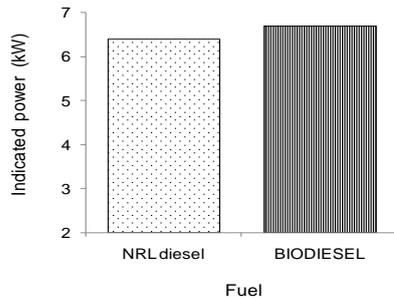
Fig. 4. IP at full load
