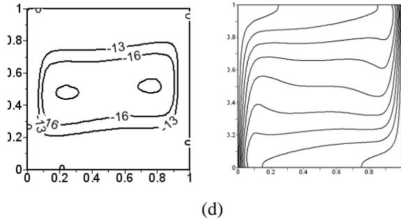
Figure 2: Streamlines and isotherms for  $Ra = 10^7$ ,  $\phi = 5\%$  for AR = (a) 0.15, (b) 0.25, (c) 0.75, (d) 1.0
