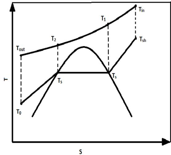
Fig. 2: T-s diagram of gas and water/steam for heat
