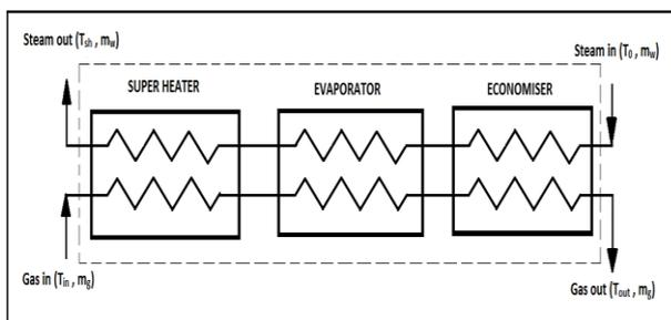
Fig.1: Schematic of the HRSG under consideration
