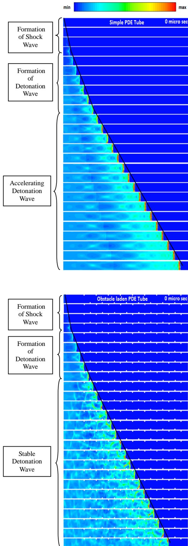
Fig.7. Pressure contour for simple and obstacle laden PDE combustor from 0 to 500  $\mu$ s
