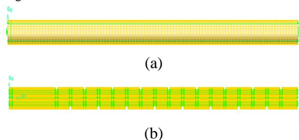
Fig.1. Discretized flow domain showing the mesh (a) Simple PDE combustor, (b) Obstacle laden PDE combustor
