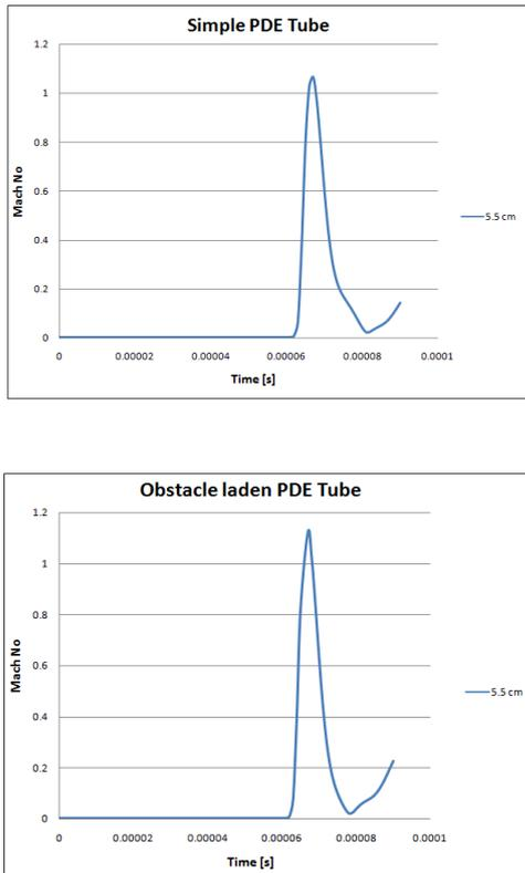
Fig.4. Mach number plot for simple and obstacle laden PDE combustor
