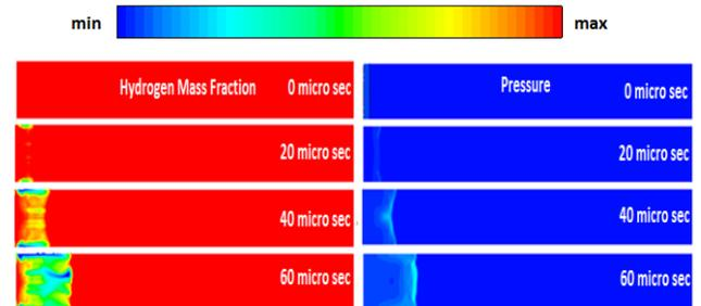
Fig.3. Hydrogen mass fraction and pressure contour plots for 50 cm long part of combustor.
