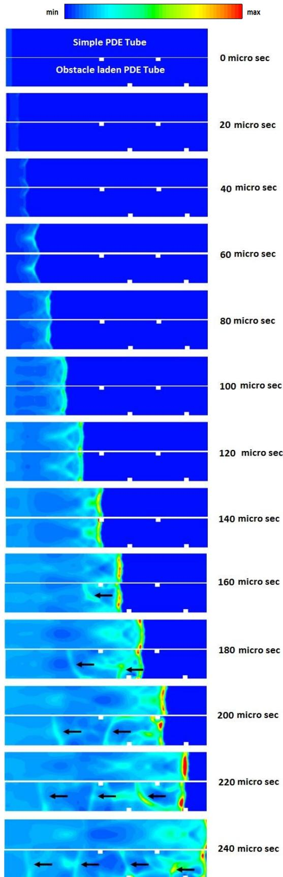
Fig.6. Pressure contour for simple and obstacle laden PDE combustor with 50 cm length
