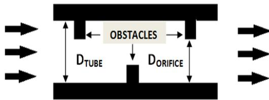
Fig.2. Schematic of obstacle laden tube
