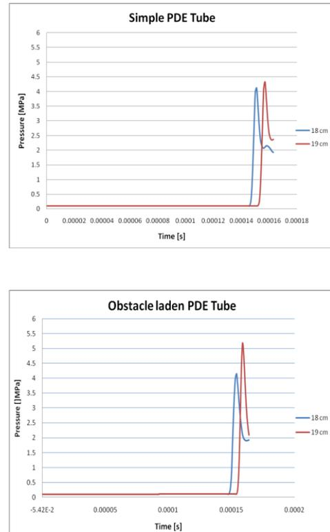
Fig.5. Pressure plot for simple and obstacle laden PDE combustor
