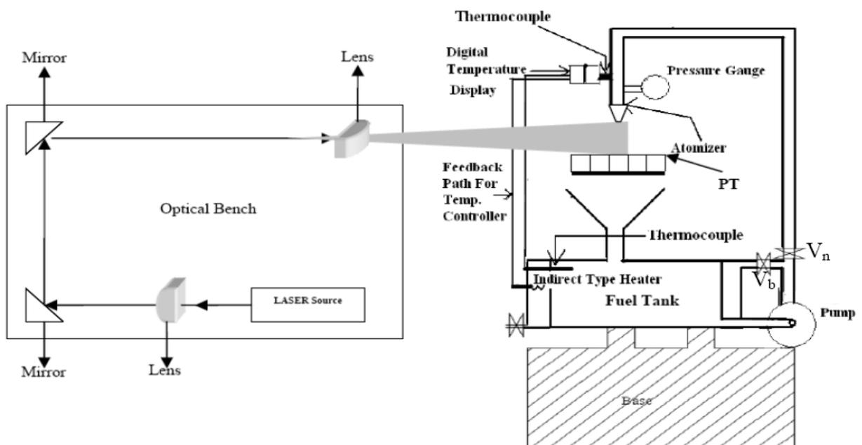
Fig.1. Schematic of the experimental set up. (PT = mechanical patternator,  $V_n$  = needle valve,  $V_b$  = ball valve)
