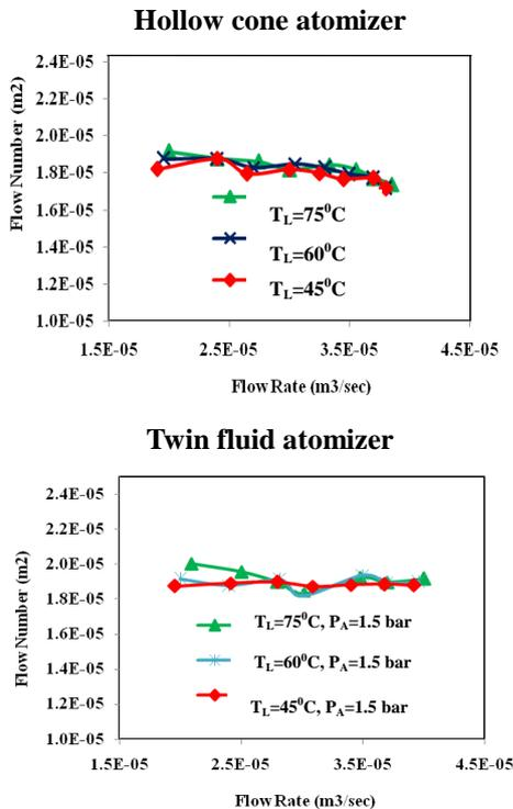
Fig.5. Variation of flow number with liquid flow rate for a hollow cone and twin fluid
