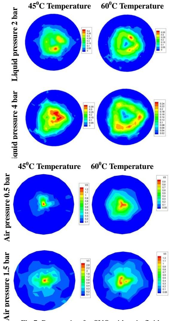
Fig.7. Patternation for SVO with twin fluid atomizer.
