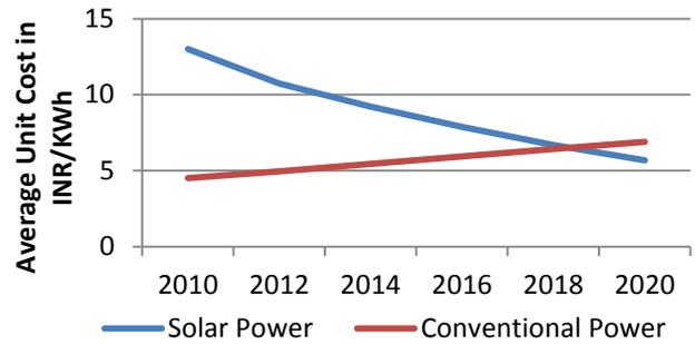
Fig 4: Variation of average unit cost in INR/KWh of Conventional Grid power and Solar power with respect to year.
