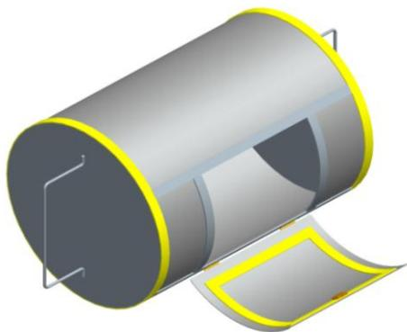
Fig.2. Charring Kiln (developed by CIAE, Bhopal)
