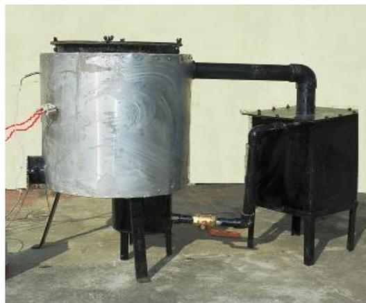
Fig.1. Vertical cylinder bio-char reactor equipped with external electrical heating systems
