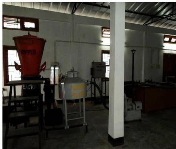
Fig.3 Woody biomass gasifier (10 kW)
