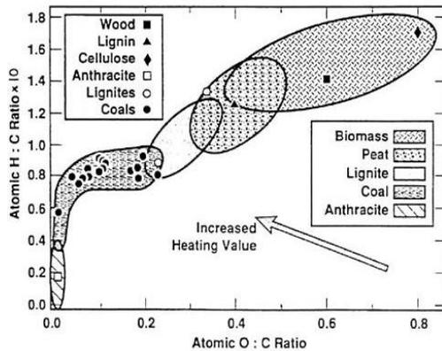
Figure 1: H/C and O/C ratio for several solid fuels (Van Krevelen diagram).
