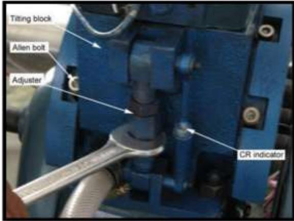
Fig. 1.2 Compression Ratio adjustments
