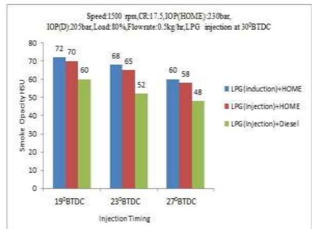
Fig. 6 Variation of smoke opacity at 80% load
