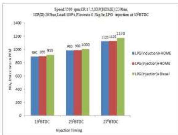
Fig. 13 Variation of NOx at 100 % load
