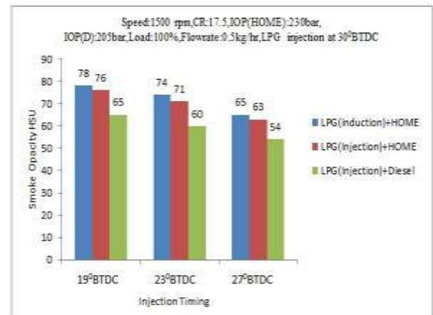
Fig. 7 Variation of smoke opacity at 100% load
