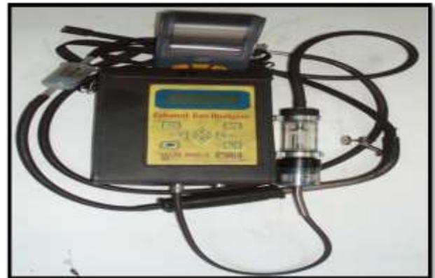
Fig. 3 Exhaust gas analyser
