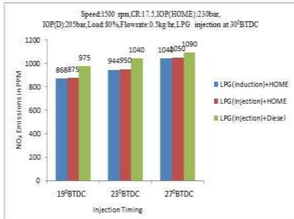
Fig. 12 Variation of NOx at 80 % load
