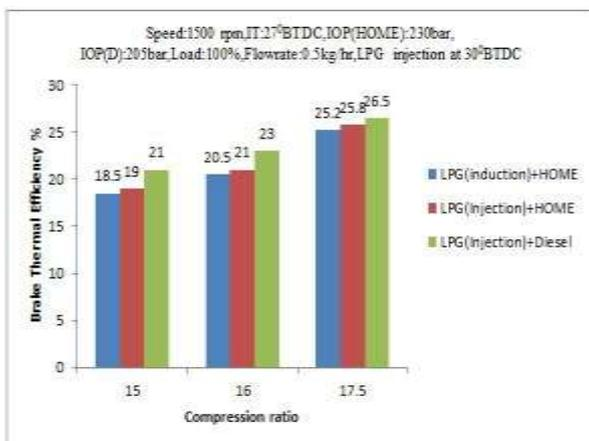
Fig.5 Variation of BTE at 100% load
