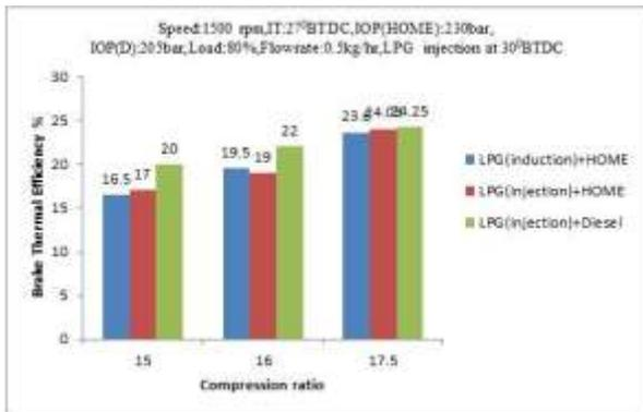
Fig. 4 Variation of BTE at 80% load
