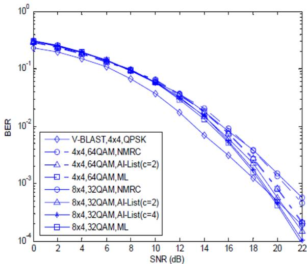
Fig 6 BER performance of SM system for the case of 8 bits/s/Hz.
