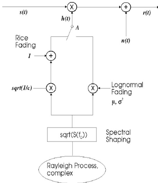
**Fig. 1** Narrowband model of a LMS channel.
