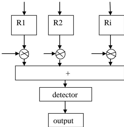
Fig 5 block diagram of MRC
