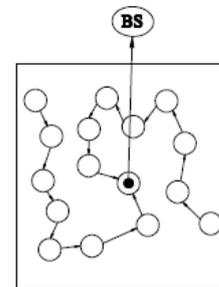
**Fig.4. A Chain-based Routing Topology**
